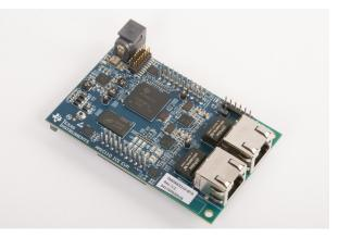
Figure 5. AMIC110 Industrial Communications Engine (ICE).
