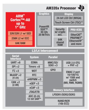
\* 1 GHz only available on 15×15 package. 13×13 is planned for 600 MHz. \*\* Use of TSC will limit available ADC channels. SED: Single error detection/parity.
