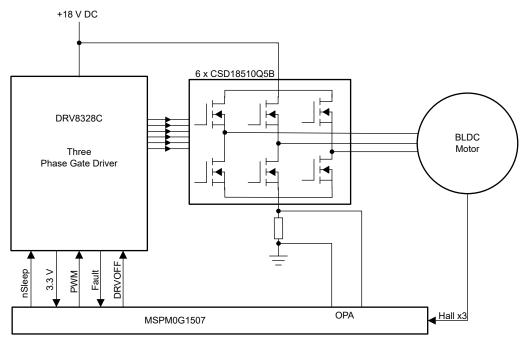
Figure 2-1. TIDA-010251 Block Diagram
