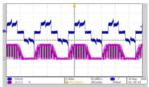
Figure 4-8. Motor Running in Open Loop
