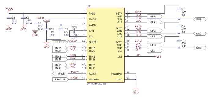
Figure 3-2. DRV8328 Gate Driver Circuit
