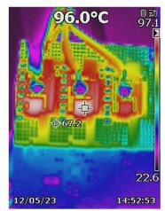
Figure 4-12. Thermal Image at 33-A<sub>RMS</sub> Winding Current, 15% Duty Cycle
