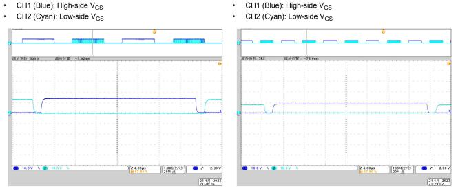
Figure 4-3. High-Side and Low-Side V<sub>GS</sub> at 18-V DC Figure 4-4. High-Side and Low-Side V<sub>GS</sub> at 5-V DC
