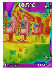
Figure 4-10. Thermal Image at 10-A<sub>RMS</sub> Winding Current, 15% Duty Cycle
