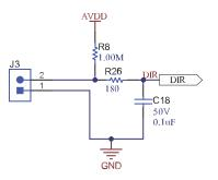
Figure 3-7. Direction Control Interface
