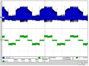
Figure 4-9. 18-V DC Input, 10-A<sub>RMS</sub> Winding Current, 15% Duty Cycle
