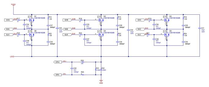
Figure 3-1. Three-Phase MOSFET Inverter
