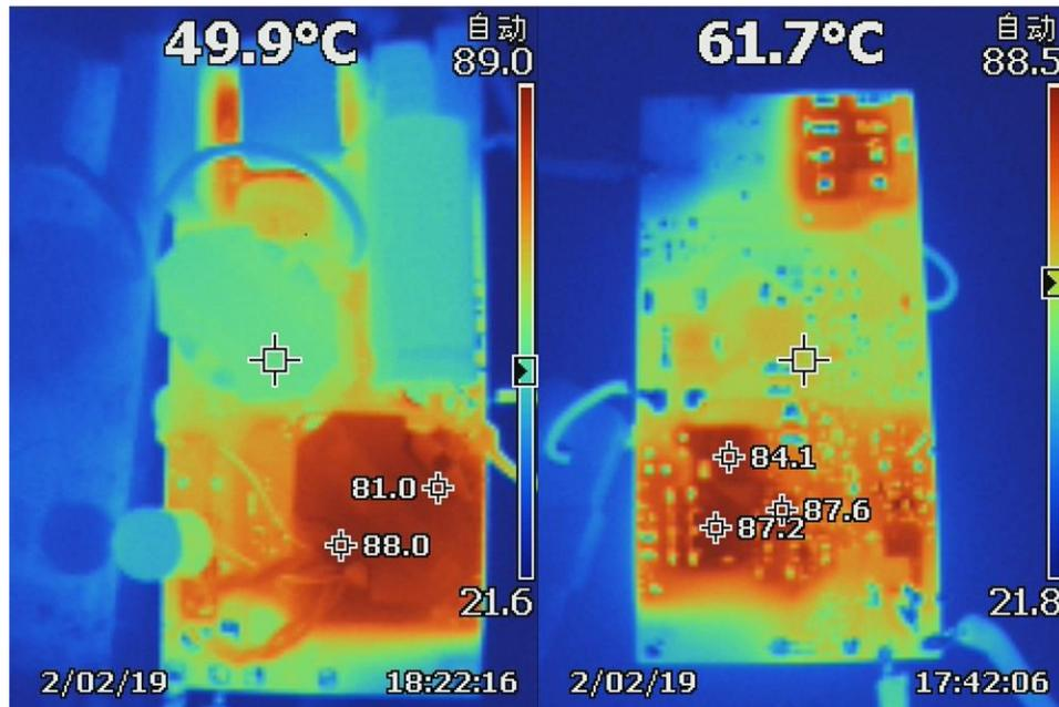
Figure 24. Thermal Image at 230-V AC, 50-Hz Input, 20-V, 5-A Output
