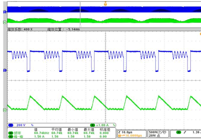
Figure 10. SW-PFC-230 VAC at Full-load
