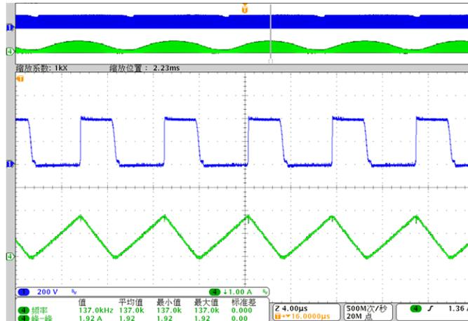
**Figure 8. PFC-115 VAC at Full-load**
