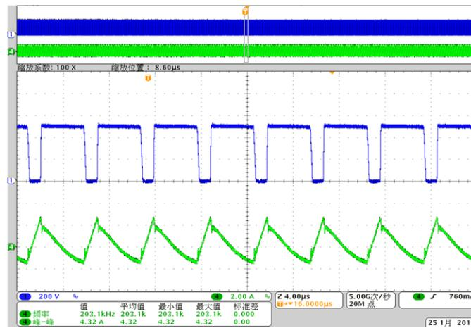
Figure 14. SW-ACF-115 VAC, 20 V<sub>OUT</sub>, 5 A
