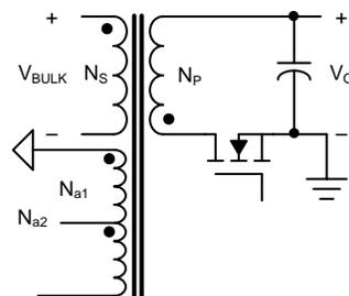
The  $N_{a1}$  winding is designed to power the devices at 5-V and 9-V outputs. Considering the voltage derating at a light load, there should be enough margin on  $V_{DD\_min}$ . Then at a 9-V output, the  $V_{DD}$  is equal to the TVS diode voltage of 16 V.  $N_{a1}$  must stay a small value to decrease the power consumption on the transistor.
