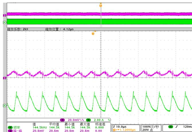
Figure 21. 115-V AC, 60-Hz Input, 20-V, 2.5-A Output
