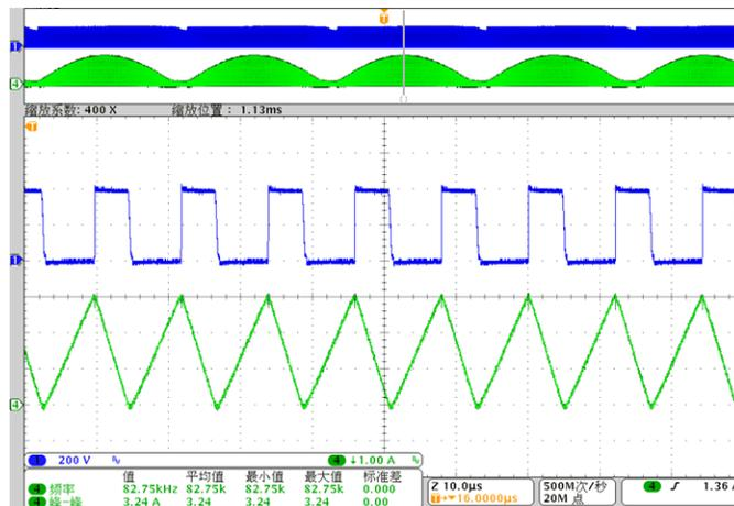
Figure 9. SW-PFC-230 VAC at Half-load
