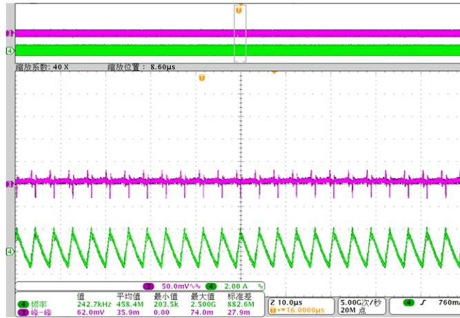
Figure 22. 115-V AC, 60-Hz Input, 20-V, 5-A Output
