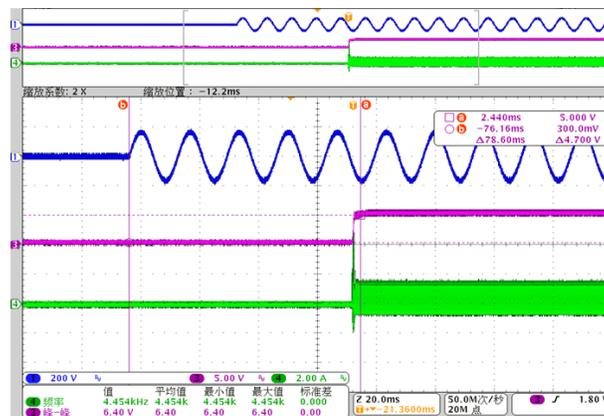
**Figure 6. Start-up Waveform at 230-V AC and 5-V, 5-A Output**
