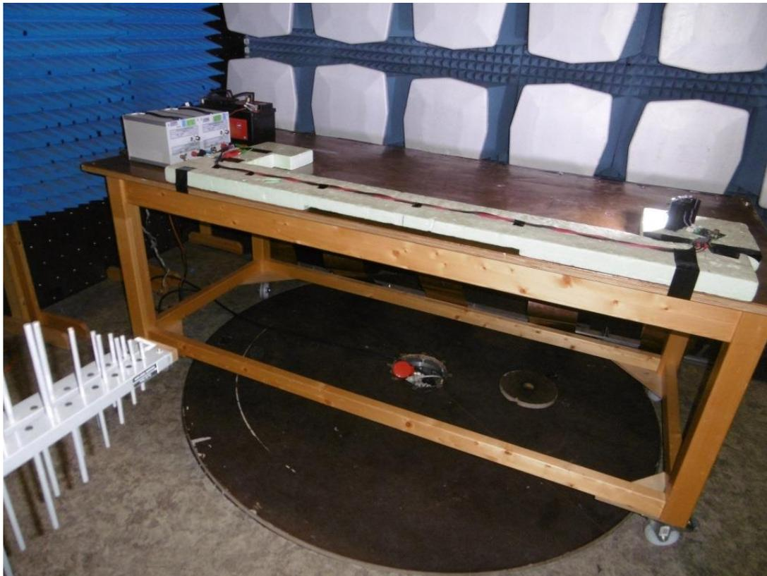
Figure 26. CISPR 25 Radiated Emissions Setup
