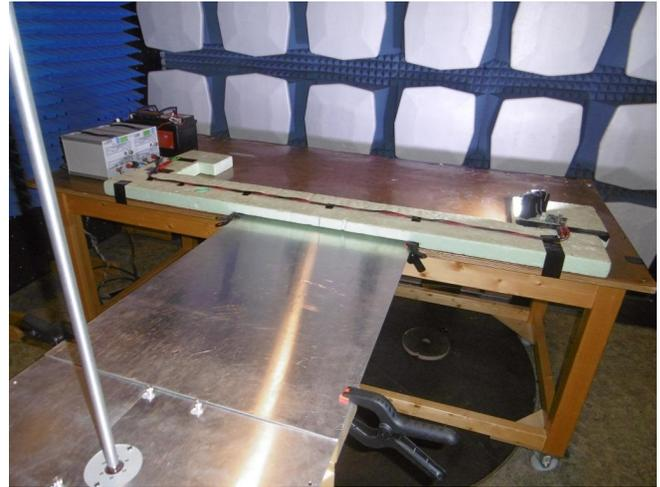
Figure 25. CISPR 25 Radiated Emissions Setup (Monopole)
