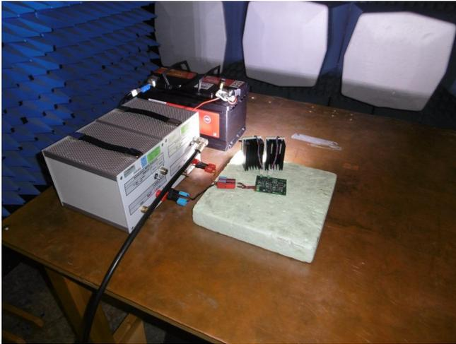
Figure 24. CISPR 25 Conducted Emissions Setup
