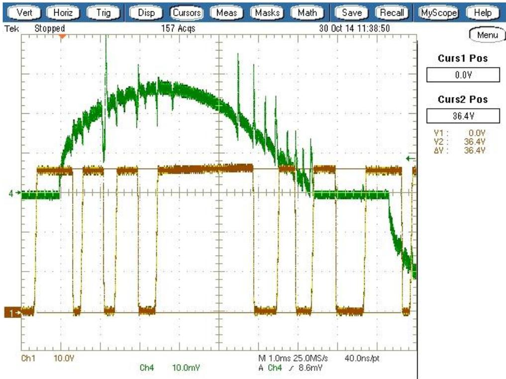
Figure 24: 3<sup>rd</sup> TPS92411 drain, 36 volts, xx1x in count sequence
