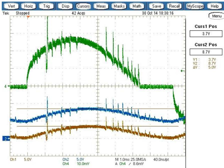
Figure 7: Voltage at current sense resistors, R26/R31 (Brown), Q3 MOSFET gate (blue)
