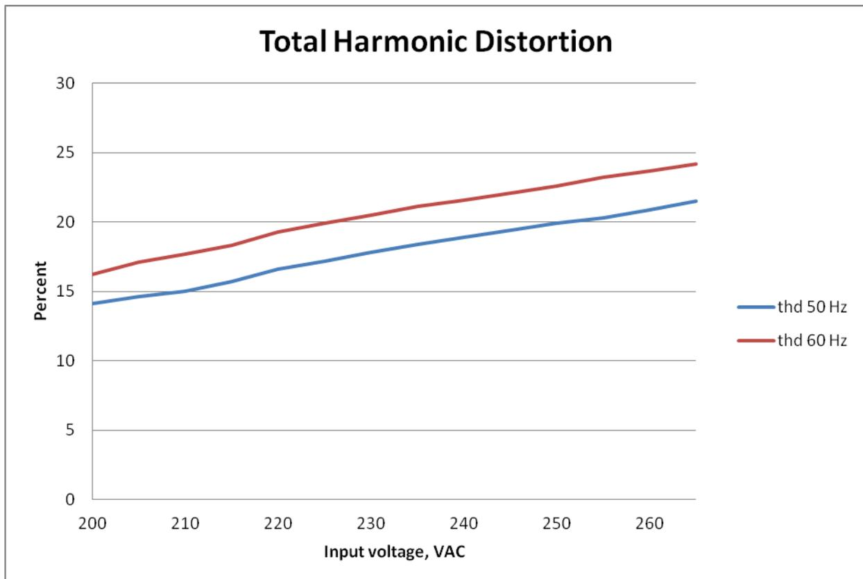
Figure 5: Total Harmonic Distortion at 50 Hz and 60 Hz, at 60 Hz line modification of line regulation circuit will lower thd level
