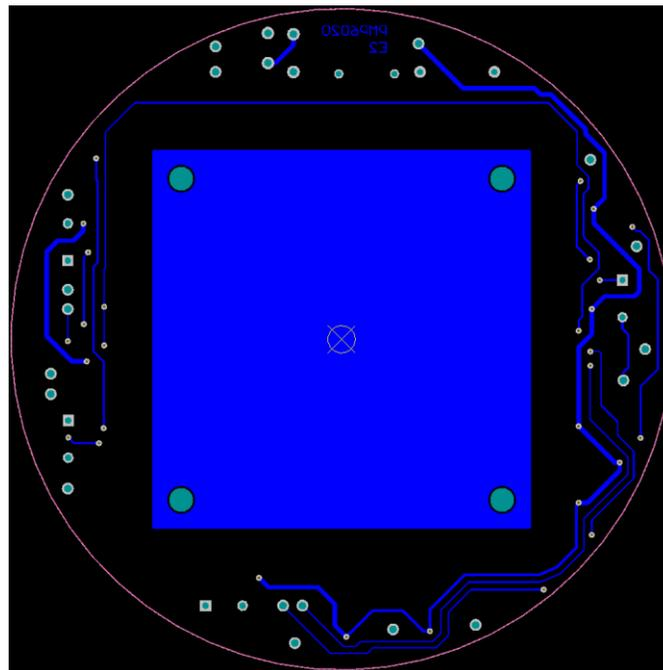
Figure 35: Bottom Layer and Bottom Overlay (Bottom view)
