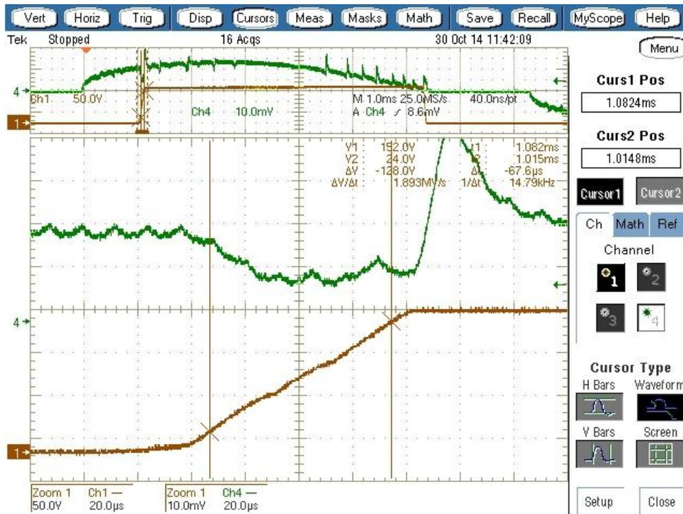
Figure 21: Drain of cascode MOSFET, open slew, 1.9V/uS
