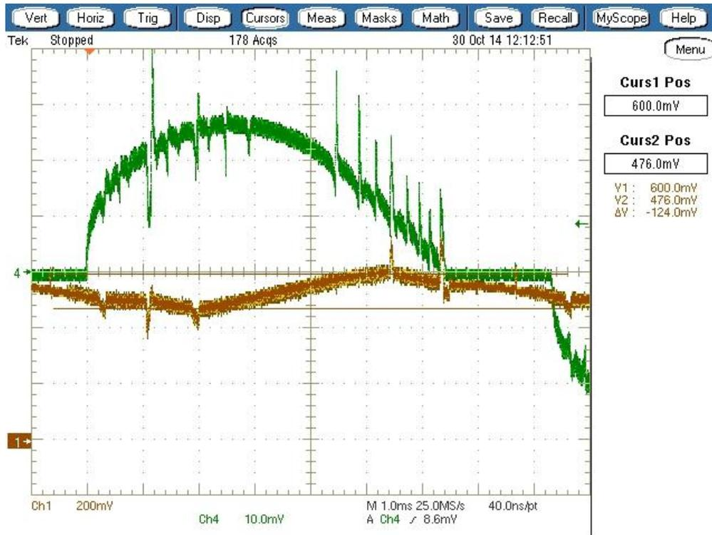
Figure 28: current ripple stack 2, 78 volt, voltage across 10 ohm resistor, approximately 23% peak to peak over average
