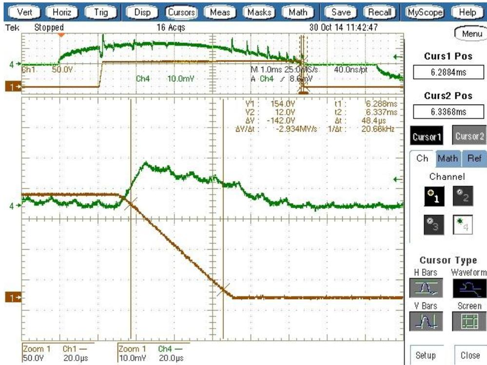
Figure 22: Drain of cascode MOSFET, close slew,  $-2.9\text{V}/\mu\text{s}$
