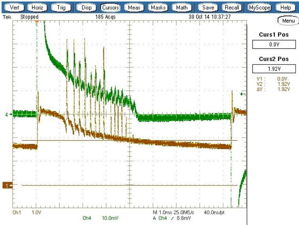
Figure 15: Current reference with DC offset, R29 (brown), shows DC offset held up by C6
