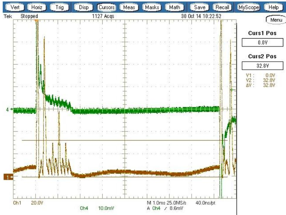
Figure 13: Current regulator drain waveform when forward phase dimming (dimmer at minimum)
