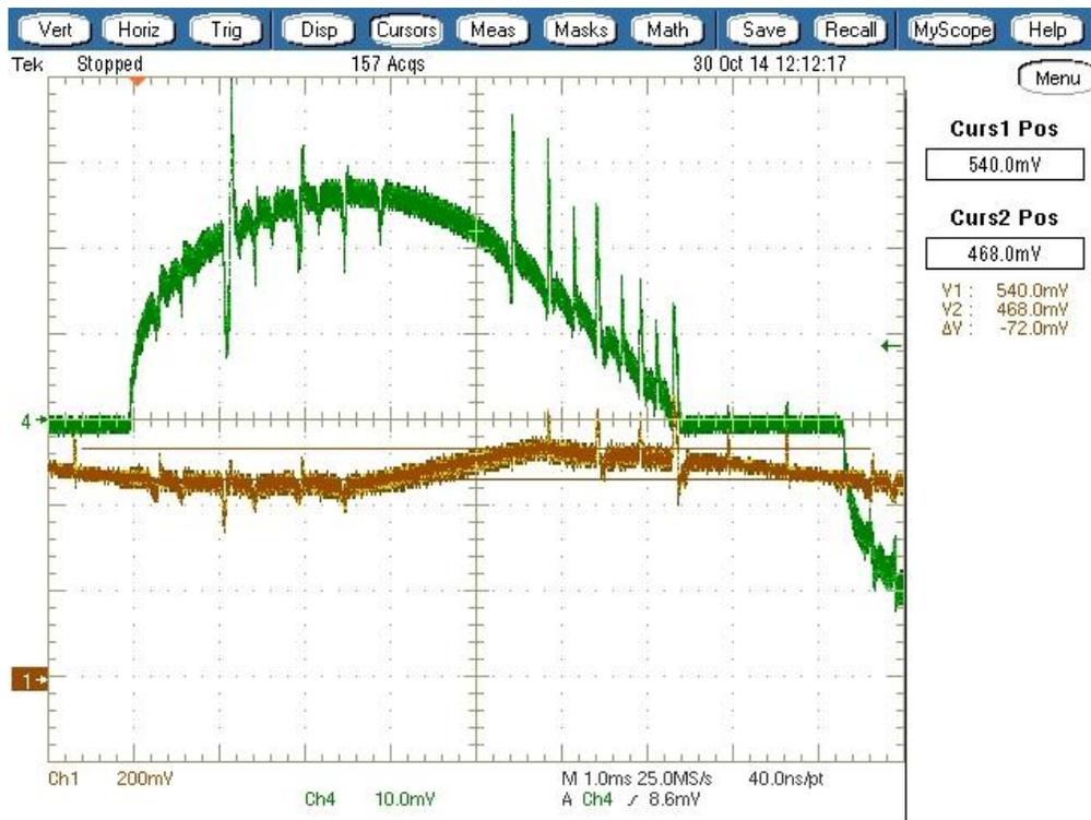
Figure 29: current ripple stack 3, 36 volt, voltage across 10 ohm resistor, approximately 14% peak to peak over average
