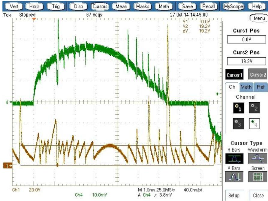
Figure 6: Current regulator drain waveform (Brown), input current (green)
