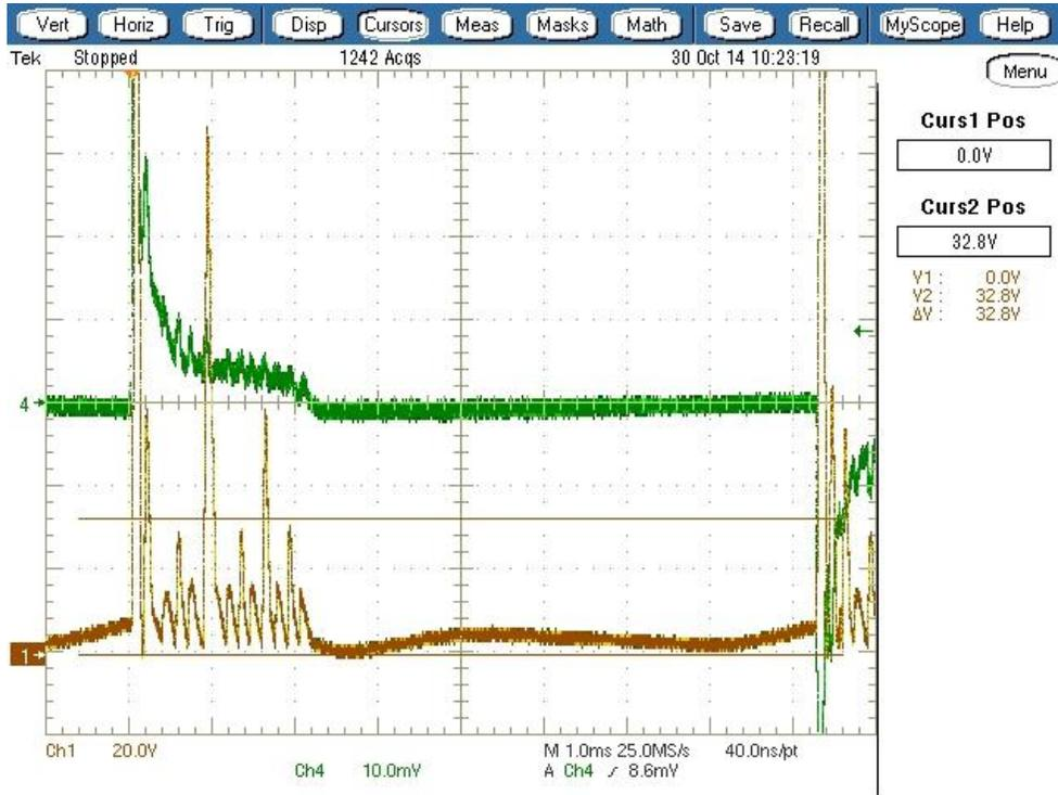
Figure 12: Current regulator drain waveform when forward phase dimming (dimmer set to about 1/4)
