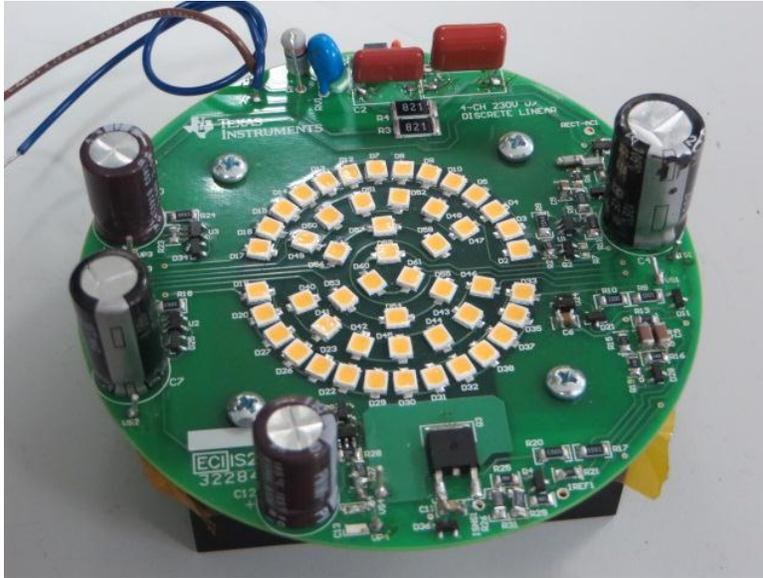
**Figure 32:** Four layer board with heat spreading planes, mounted to ½-brick heatsink for testing
