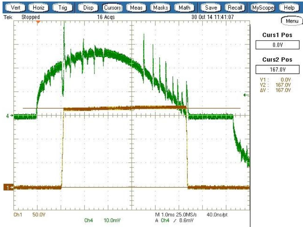
Figure 20: Drain of cascode MOSFET showing slew control, turn-on faster than turn-off. 1<sup>st</sup> stack, 168 volt, 1xxx in count sequence
