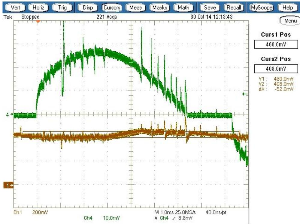
**Figure 30: current ripple stack 4, 18 volt, voltage across 10 ohm resistor, approximately 12% peak to peak over average**
