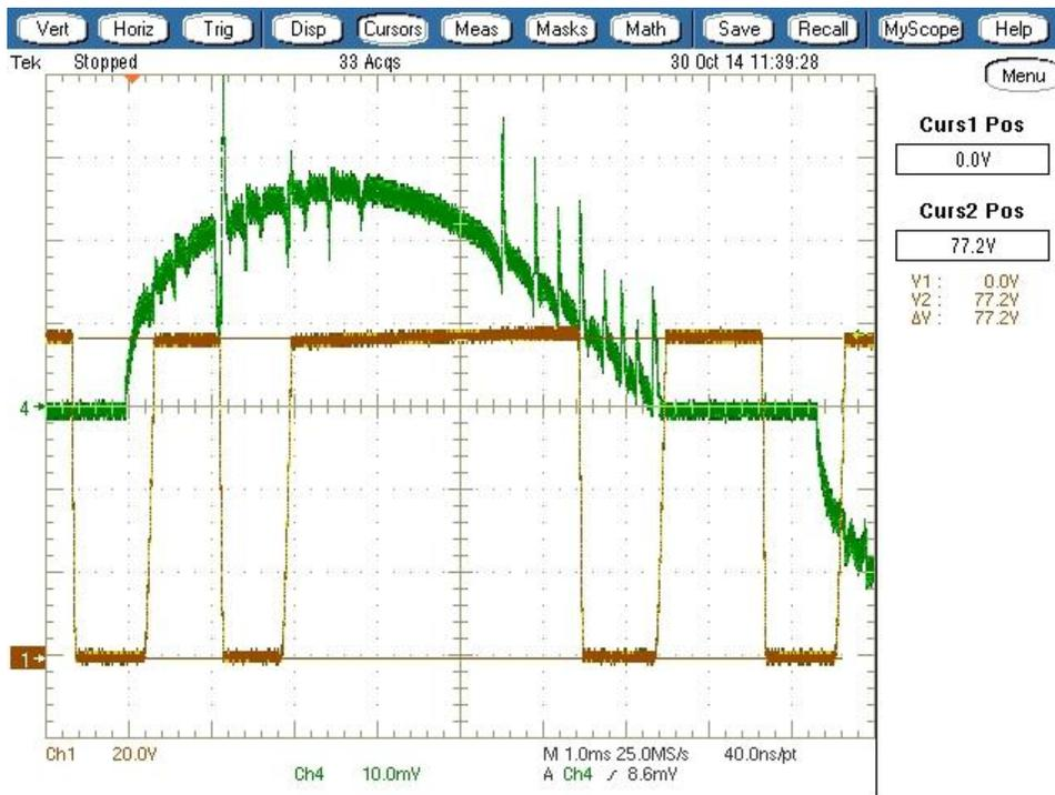
Figure 23: 2<sup>nd</sup> TPS92411 drain, 78 volt stack, x1xx in count sequence
