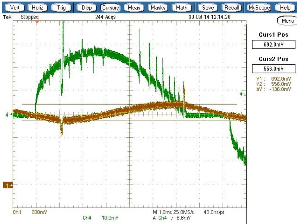
Figure 27: current ripple stack 1, 168 volt, voltage across 10 ohm resistor, approximately 22% peak to peak over average
