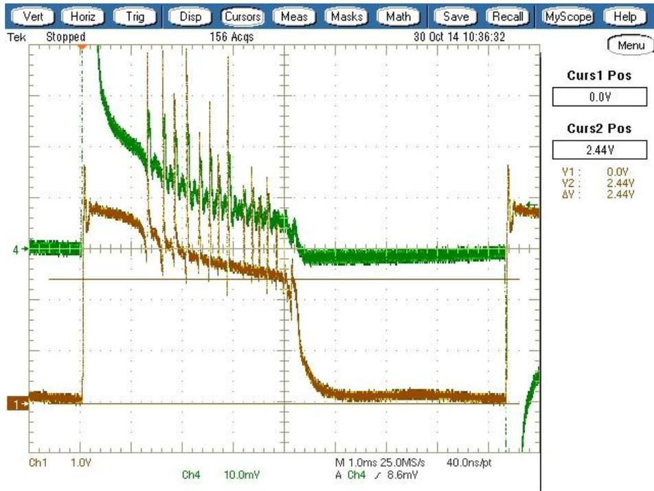
Figure 16: Current sense voltage while forward phase dimming, R15 (brown)
