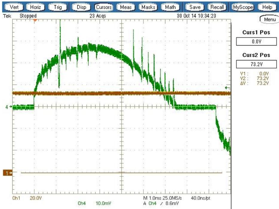
Figure 17: Input averaging voltage used for line regulation, D28 (brown)
