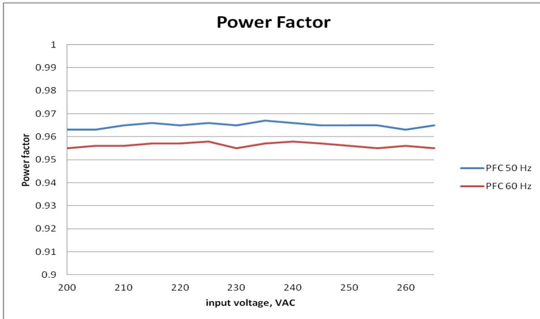
Figure 4: Power factor correction at 50 Hz and 60 Hz
