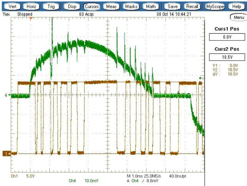
Figure 25: 4<sup>th</sup> TPS92411 drain, 18 volts, xxx1 in count sequence
