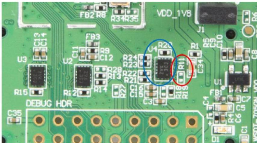
**Figure 14. R11 DNI to Enable Audio Features**
