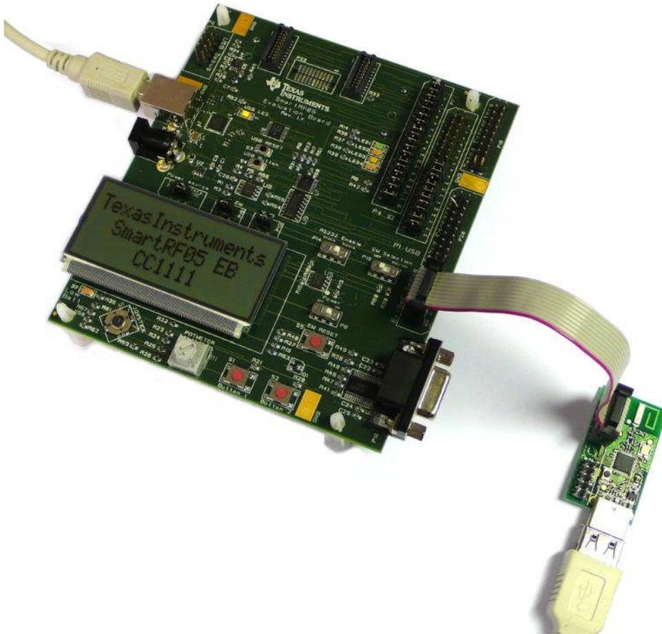
**Figure 8 - SmartRF05EB connected to a CC1111 USB Dongle**
