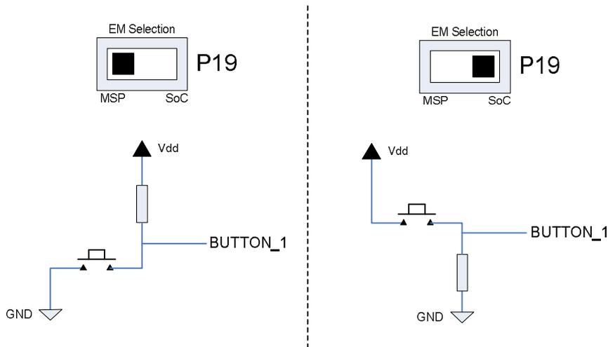
**Figure 21 - Switch P19 effect on Button 1**
