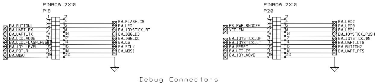
Debug connectors mirror EM connectors with a few exceptions. Exceptions: Pins 1, 2 and 3 left unconnected, GND connected to pin 20. Reason for exception is to be able to connect an Agilent logic analyzer probe directly to the debug connector.
