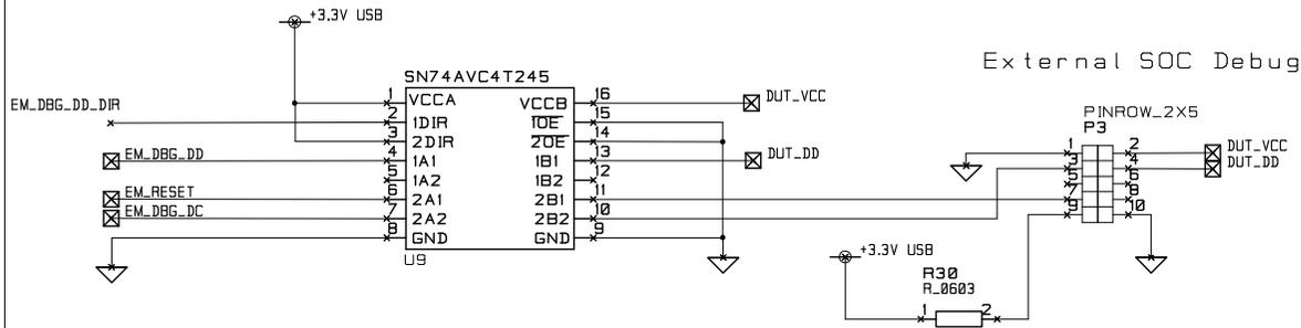
Mount 0 ohm resistor in position R30 to power DUT from +3.3V USB through connector P3
