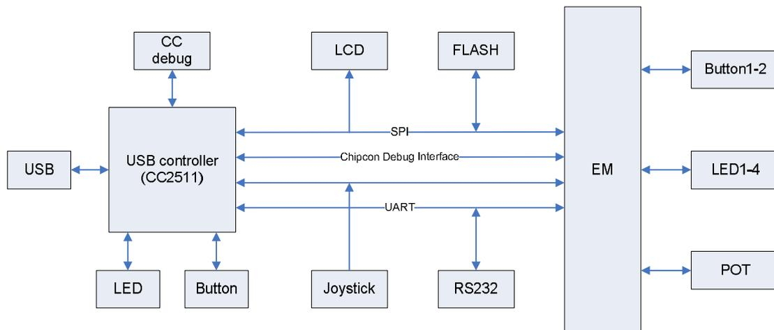
**Figure 9 - SmartRF05EB architecture**
