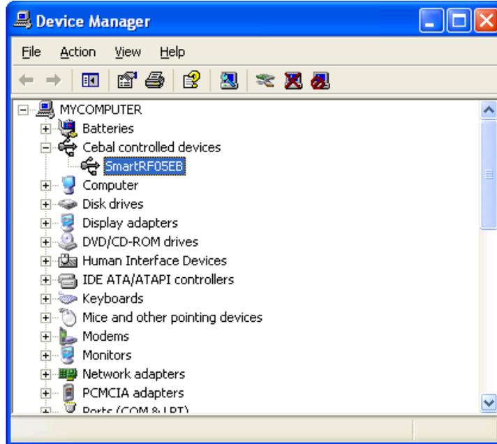
**Figure 5 - Properly installed SmartRF05EB software (Windows XP)**
