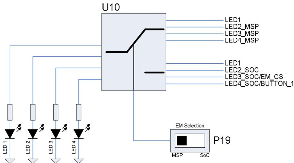
Figure 20 - Switch P19 effect on LED 1-4
