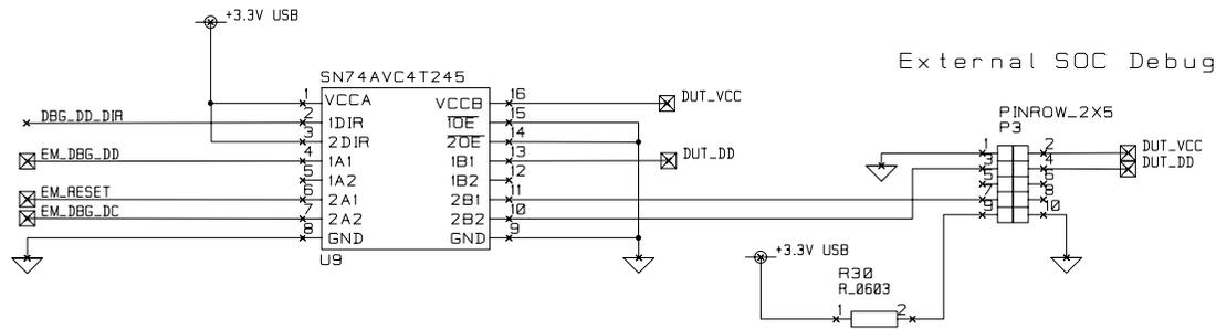
Mount 0 ohm resistor in position R30 to power DUT from +3.3V USB through connector P3
