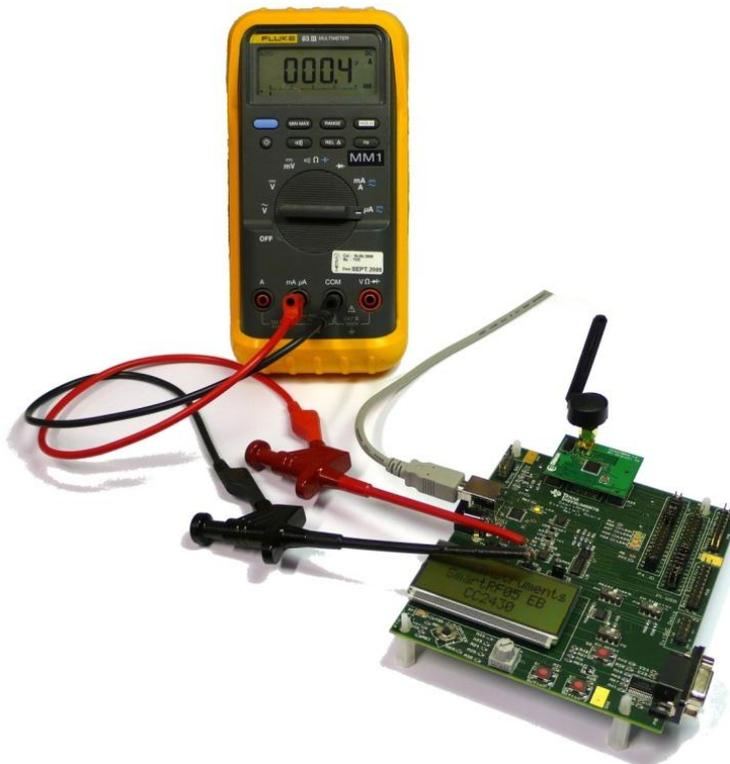
Figure 14 - Current measurement set-up
