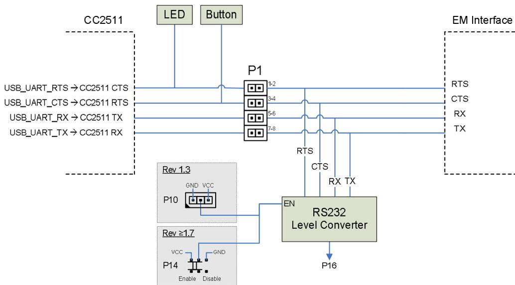
**Figure 11 - UART RS232 signals and jumpers**
