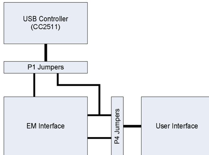
**Figure 18 - Basic signal flow on the evaluation board**
