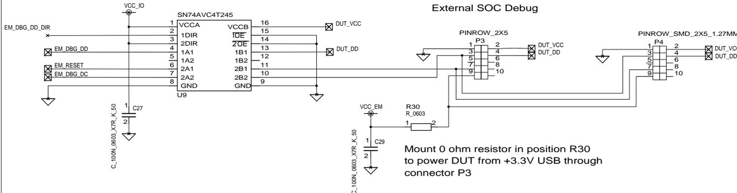
Mount 0 ohm resistor in position R30 to power DUT from +3.3V USB through connector P3
