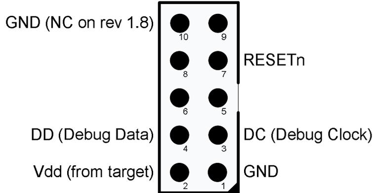
Figure 15 - SmartRF05EB External SoC Debug Connector
