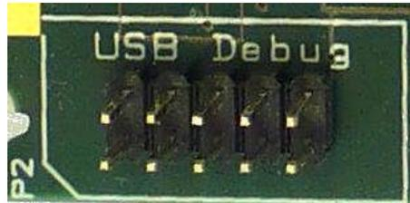
**Figure 23 - USB controller debug connector**
