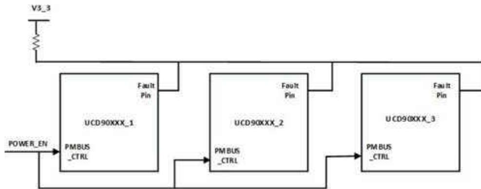
**Figure 1. Example Using a Typical Fault Pin**
