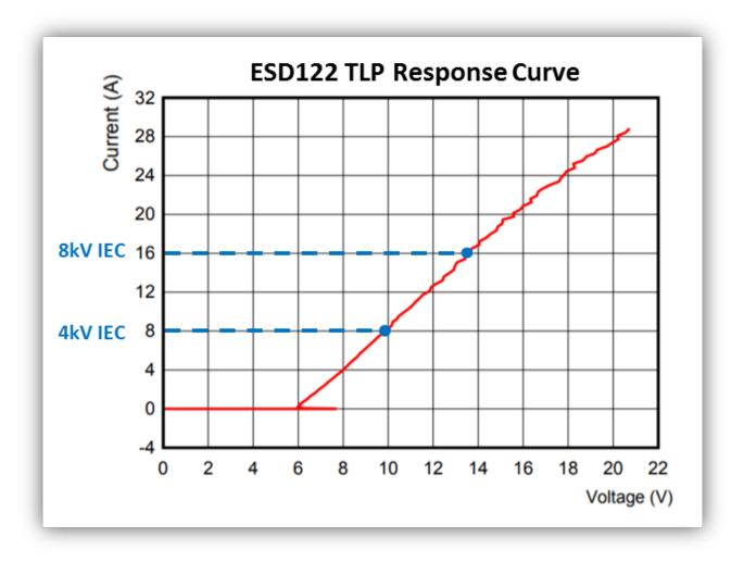
Figure 2. TLP Response Curve for the ESD122
