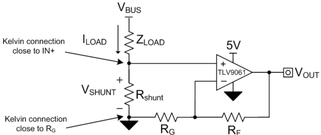
**Figure 4. Schematic Representation of a Proper Layout**
