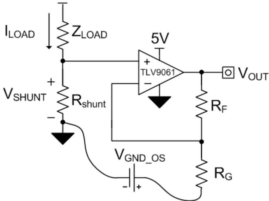
**Figure 3. Voltage Differences on the Ground Plane**
