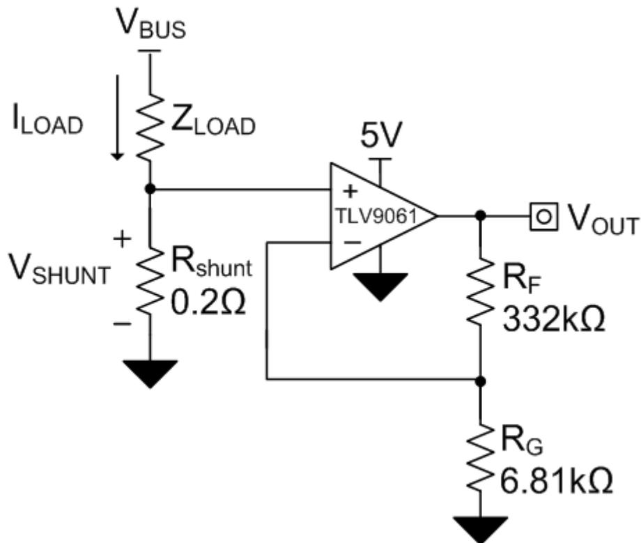
**Figure 1. Low-side Current-sensing Schematic**
