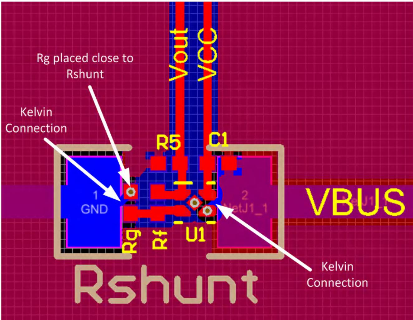
**Figure 5. Proper PCB Layout for Low-side Current Sensing**
