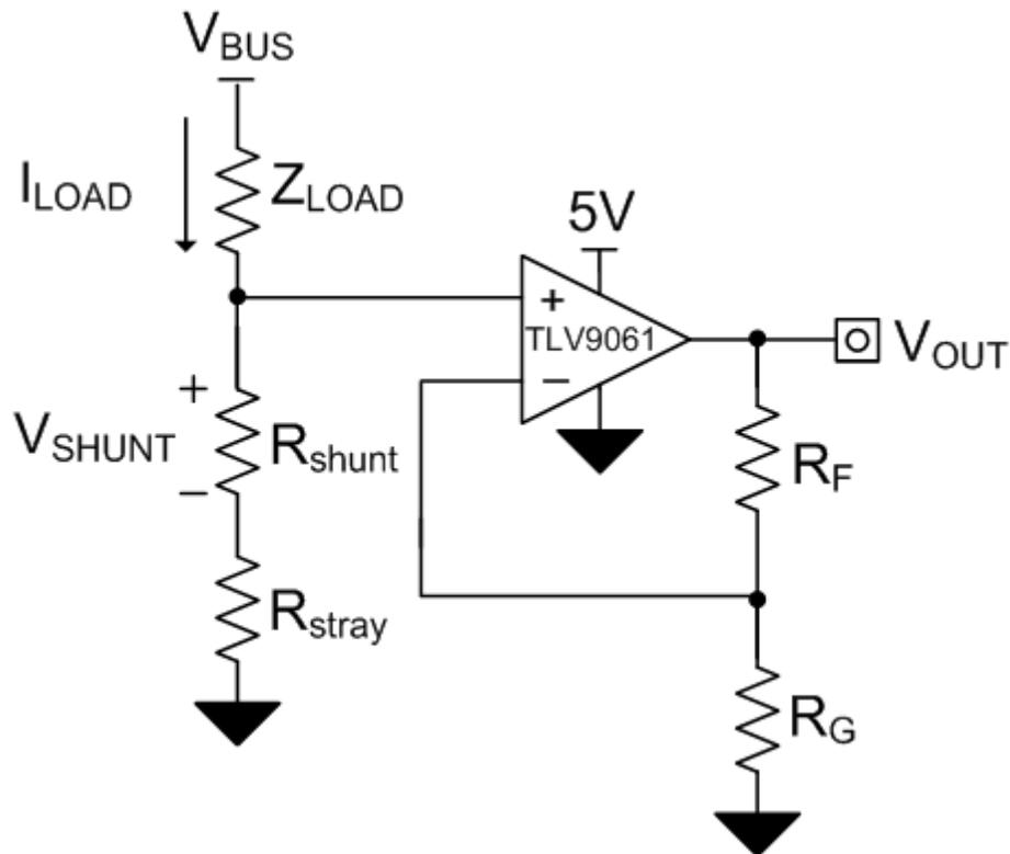
**Figure 2. Stray Resistance in Series with  $R_{shunt}$**
