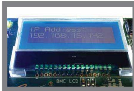
**5** Note the IP address displayed on LCD screen. Enter this address into a web browser connected to the same network as the EVM.
