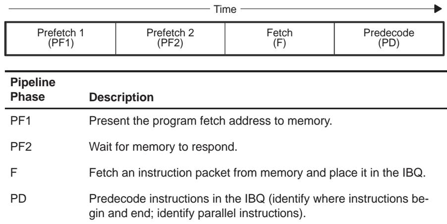
Figure 4–9. Second Segment of the Pipeline (Execution Pipeline)
