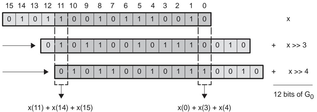
Example 7–3 shows an implementation of the output bit streams for the convolutional encoder of Figure 7–3.
