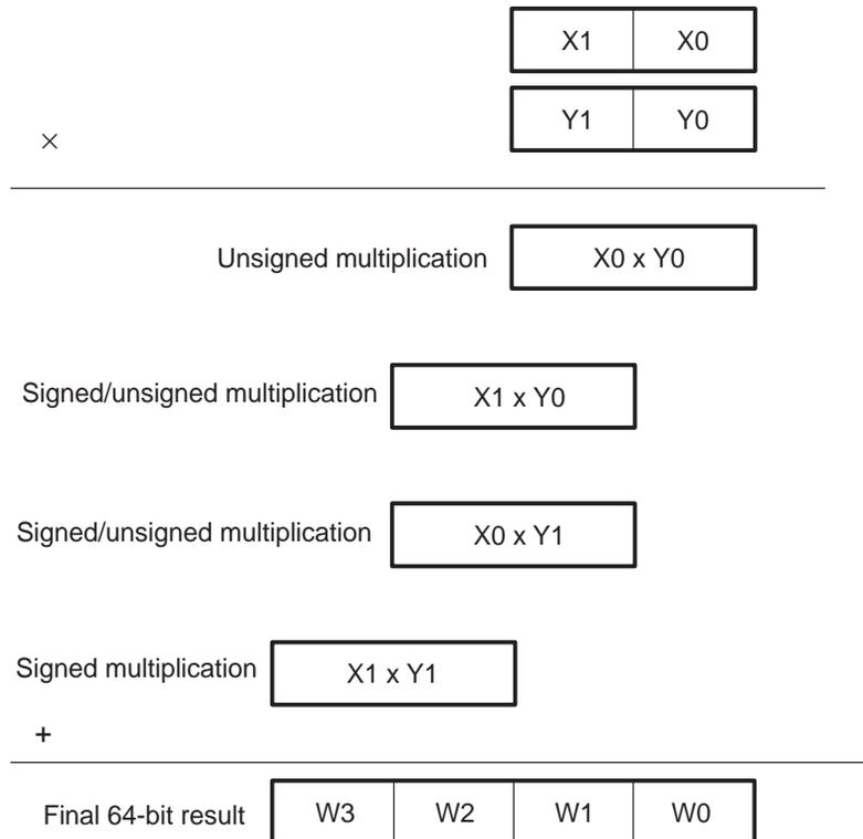
Example 5–8 shows that a multiplication of two 32-bit integer numbers requires one multiplication, two multiply/accumulate/shift operations, and a multiply/accumulate operation. The product is a 64-bit integer number. Example 5–9 shows a fractional multiplication. The operands are in Q31 format, while the product is in Q31 format.
