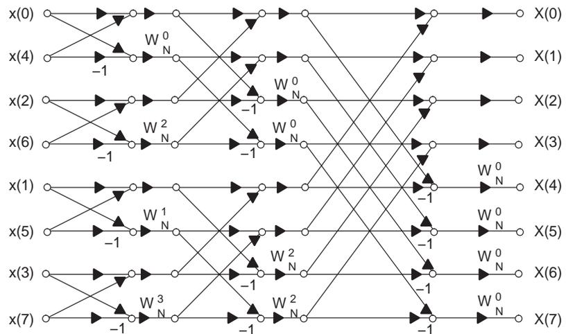
Consider a complex FFT of size  $N$  (that is, an FFT with an input vector that contains  $N$  complex numbers). You can bit-reverse either the input or the output vectors by executing the following steps:
