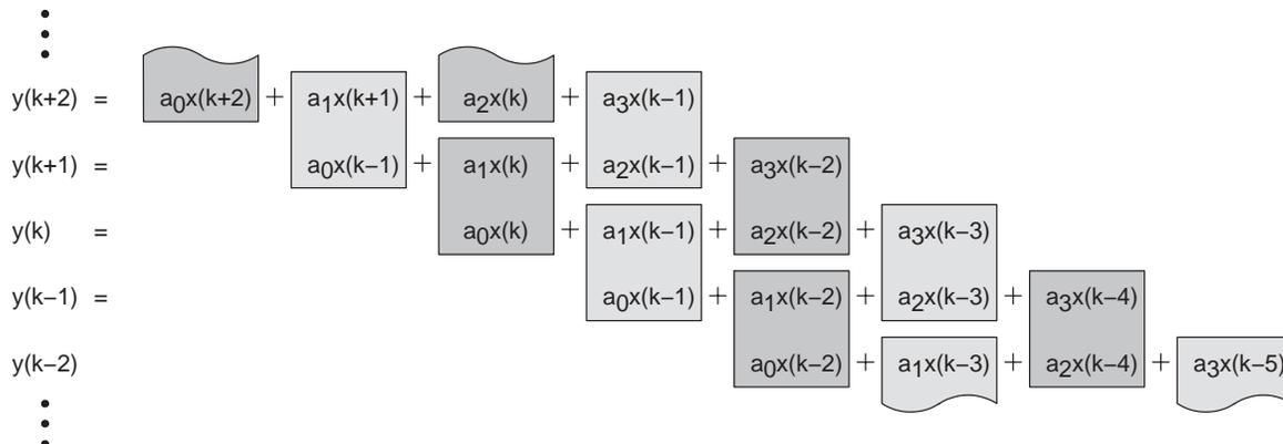
Notice that two separate running sums are maintained, one with partial products for the current time step, the other with pre-computed terms for the next time step. At the next time step, the pre-computed running sum becomes the current running sum, and a new pre-computed running sum is started from zero. At the end of each sample period, the current running sum contains the current filter output, which can be dispatched as required by the application.
