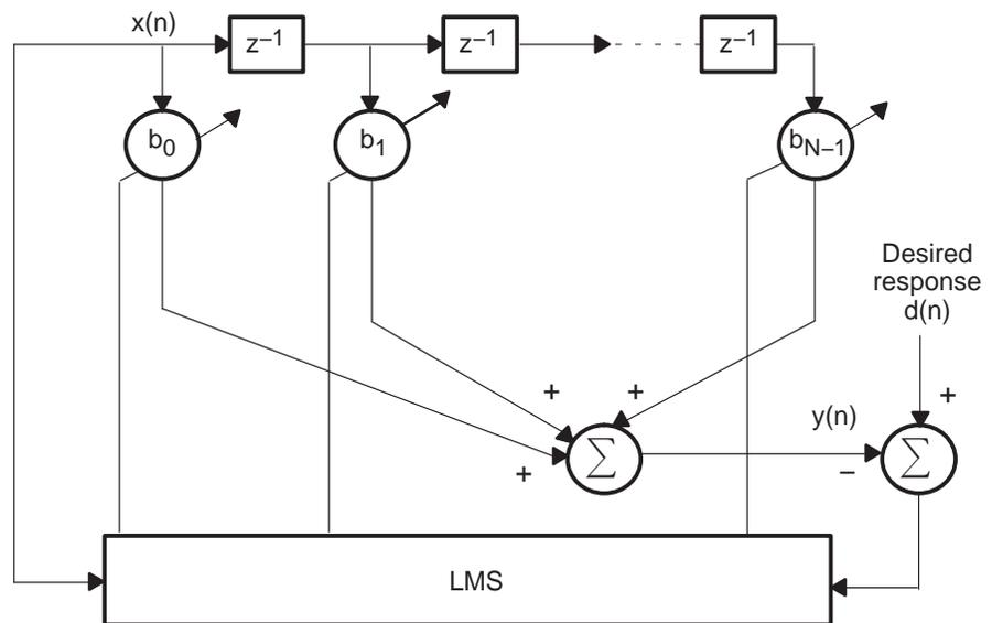
Two common algorithms employed for least mean squares adaptation are the non-delayed LMS and the delayed LMS algorithm. When compared to non-delayed LMS, the more widely used delayed LMS algorithm has the advantage of greater computational efficiency at the expense of slightly relaxed convergence properties. Therefore, section 7.2.1 describes only the delayed LMS algorithm.
