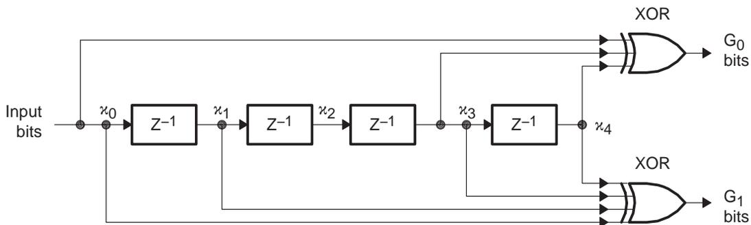
The C55x DSP creates the output streams ( $G_0$  and  $G_1$ ) by XORing the shifted input stream (see Figure 7–4).
