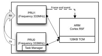
Figure 2-5. PRU Direct Mode System Block Diagram
