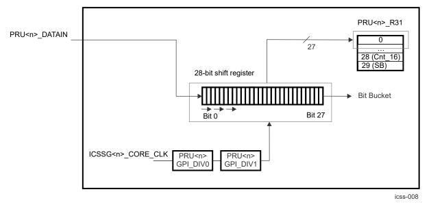
Figure 2-8. PRU R30 (GPO) Shift Out Mode Block Diagram
