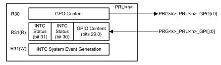
Figure 2-1. PRU GPIO Interface
