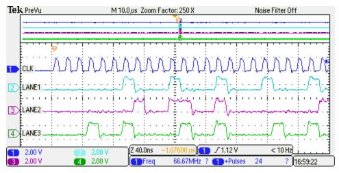
Figure 3-5. 4-Lane Parallel Data Transmission
