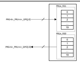
Figure 2-2. PRU Direct Input and Output Mode Block Diagram
