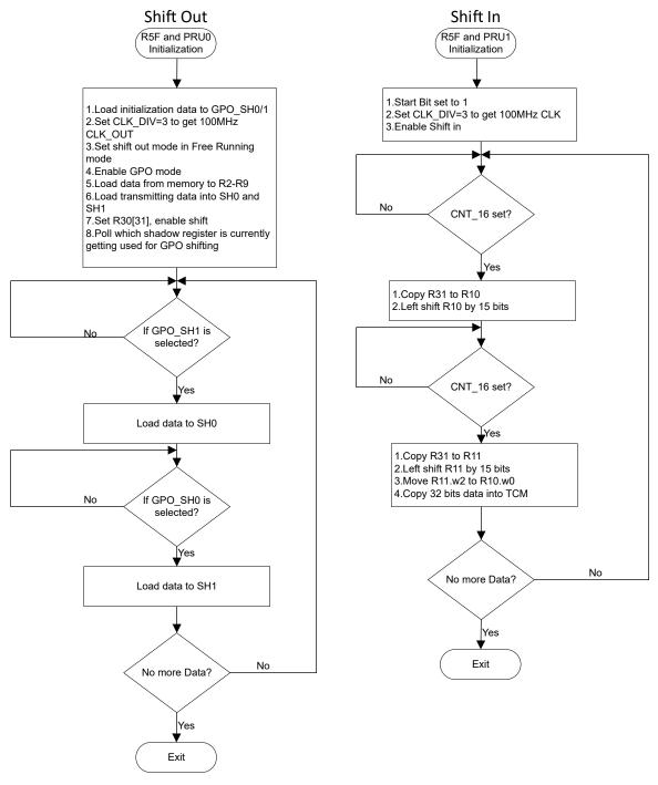
Figure 2-9. PRU Shift Out and In Programming Work Flow
