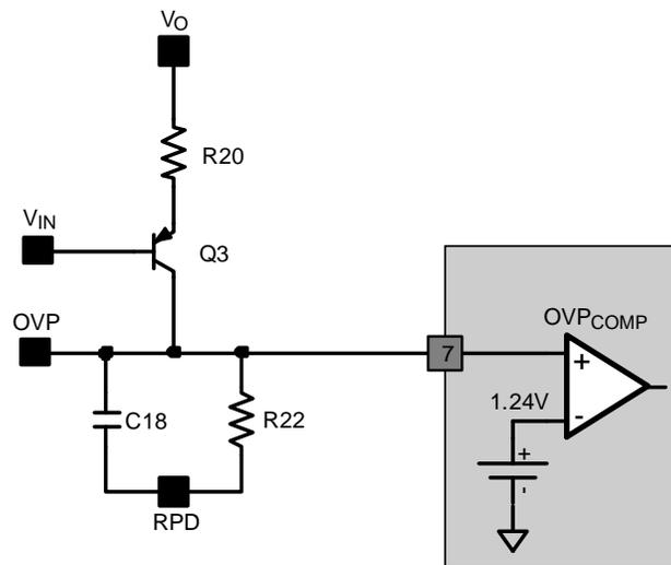
**Figure 8. OVP Circuit**
