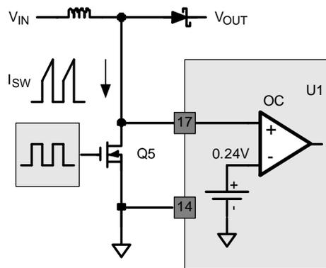
Figure 5. MOSFET  $R_{DS(ON)}$  Sensing Configuration
