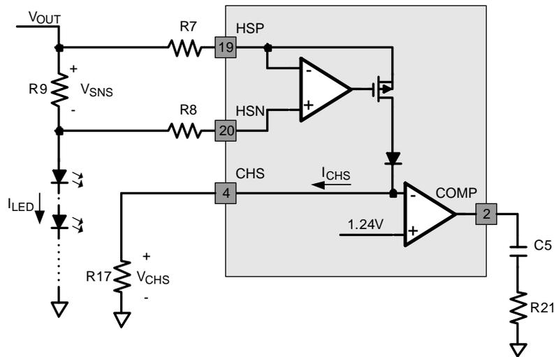
**Figure 2. High-Side Sensing Circuit**
