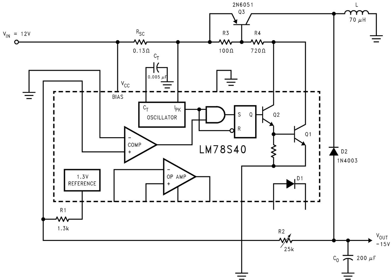
**Figure 14. Inverting Regulator**
