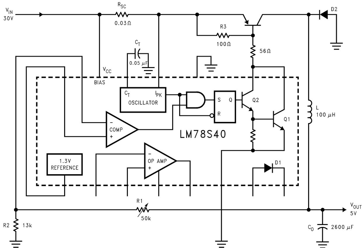
Figure 13. Modified Step-Down Regulator with 5A, 5V Output
