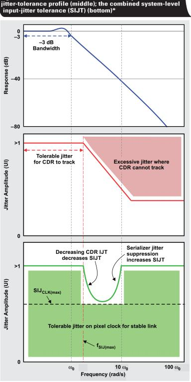
Figure 6. Serializer PLL transfer function (top); deserializer
