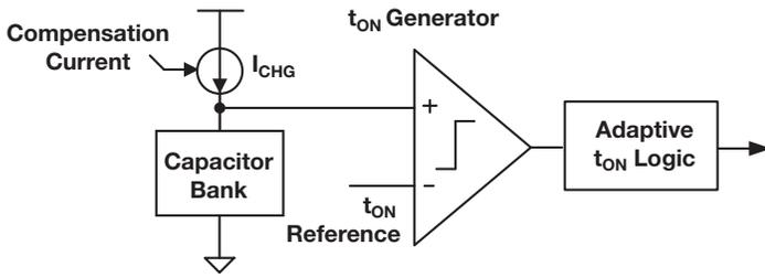
Figure 2: Block diagram of adaptive on-time generation.
