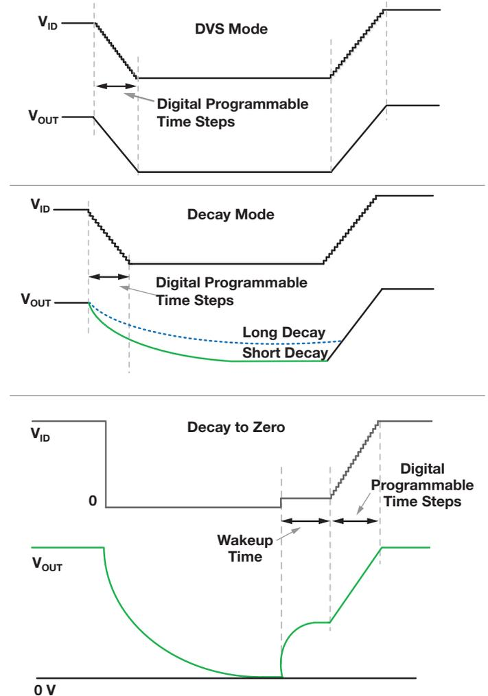
Figure 5: DVS- and decay-mode waveforms.
