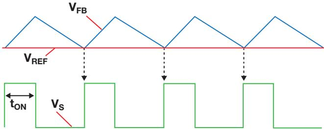
Figure 3: Switching waveforms for adaptive on-time control.
