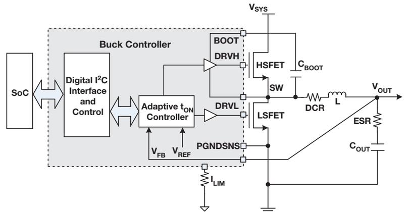
Figure 1: Block diagram of a buck controller in the TPS65086x.
