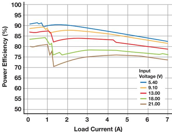
Figure 4: Buck controller power efficiency vs. load current.
