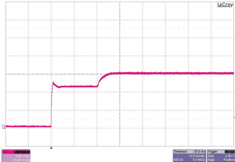
The photo below shows the 15V output voltage startup waveforms after the application of 4.5Vdc in. The output was unloaded.
