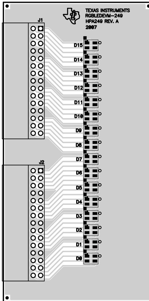
Figure 14. Assembly Layer
