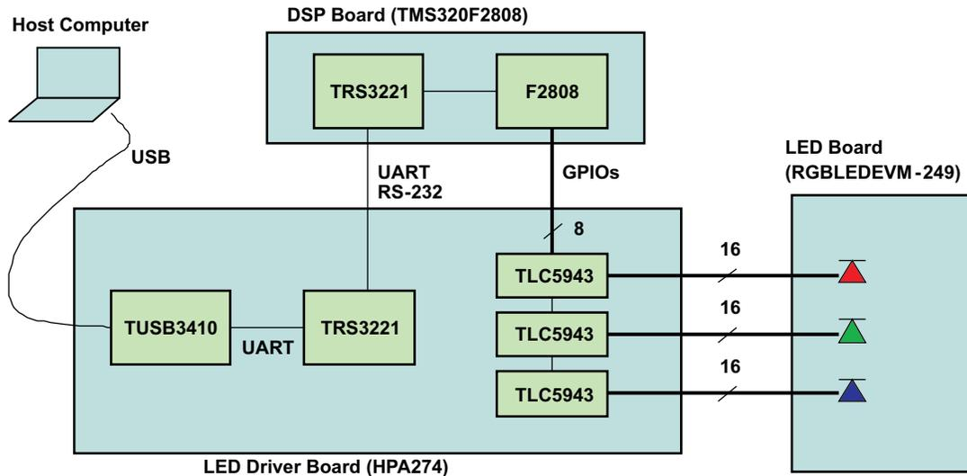
Figure 1. Board Connections
