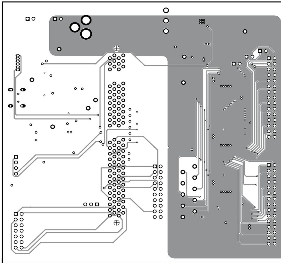
Figure 11. Layer 2 Routing
