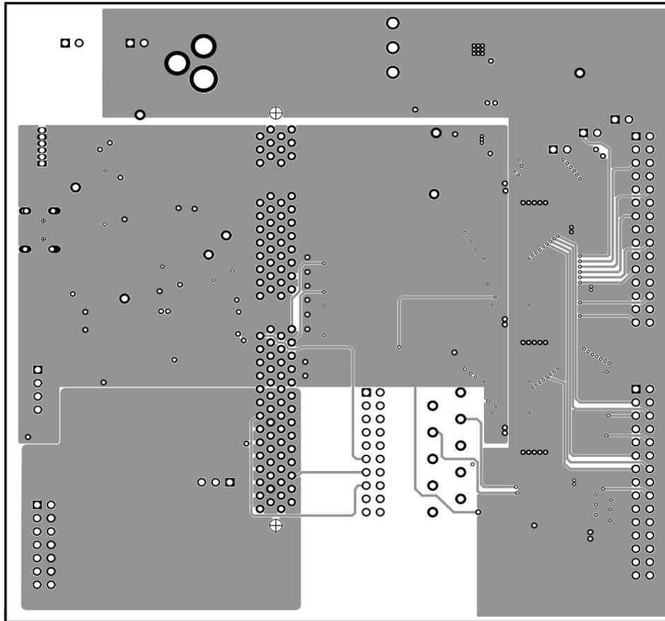
**Figure 12. Layer 3 Routing**
