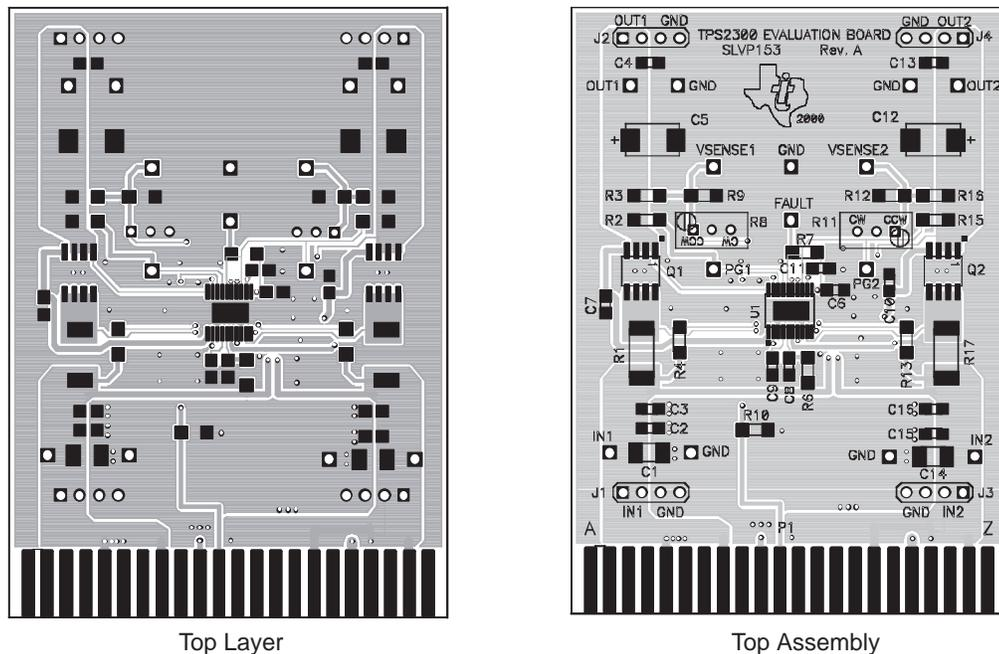
Figure 1–4. Top Layer of the Interface Card, and Placement of Components
