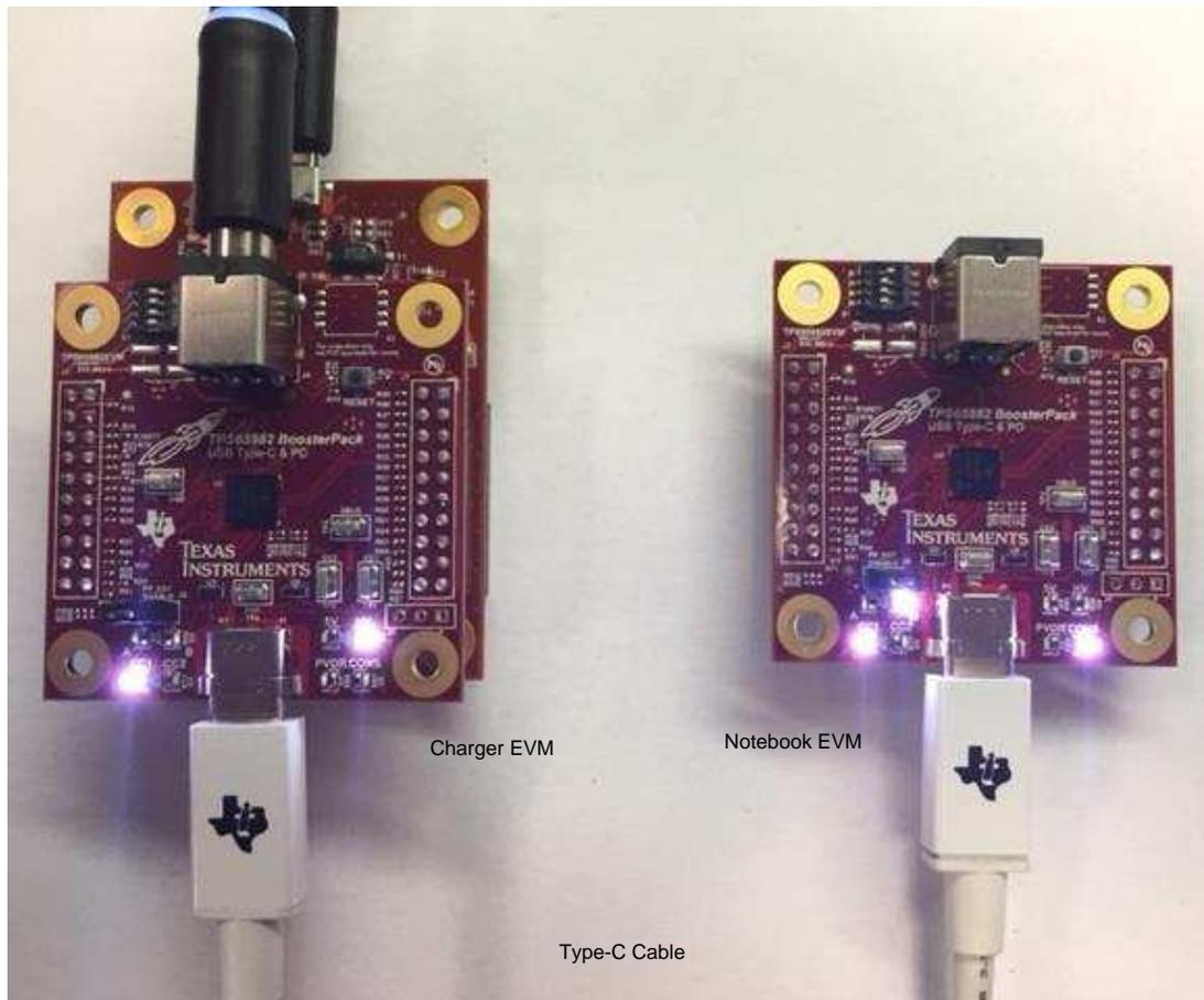
**Figure 28. Type-C and PD System Demo**
