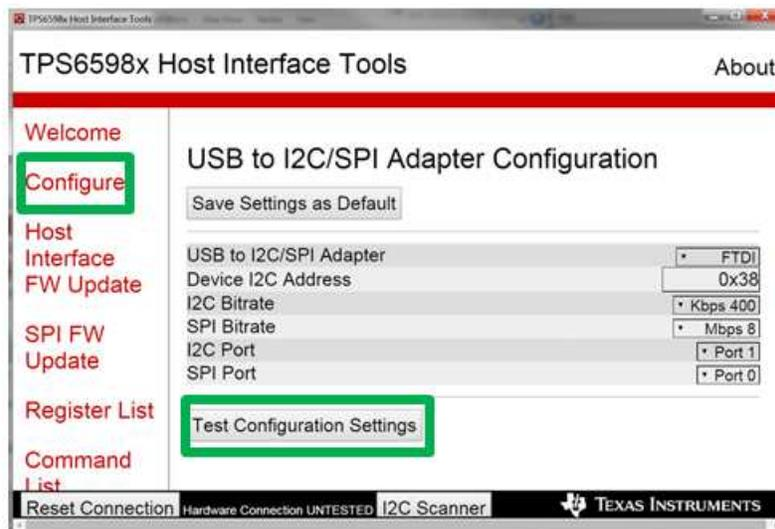
Figure 6. Configure Tab in TPS6598x Utilities GUI
