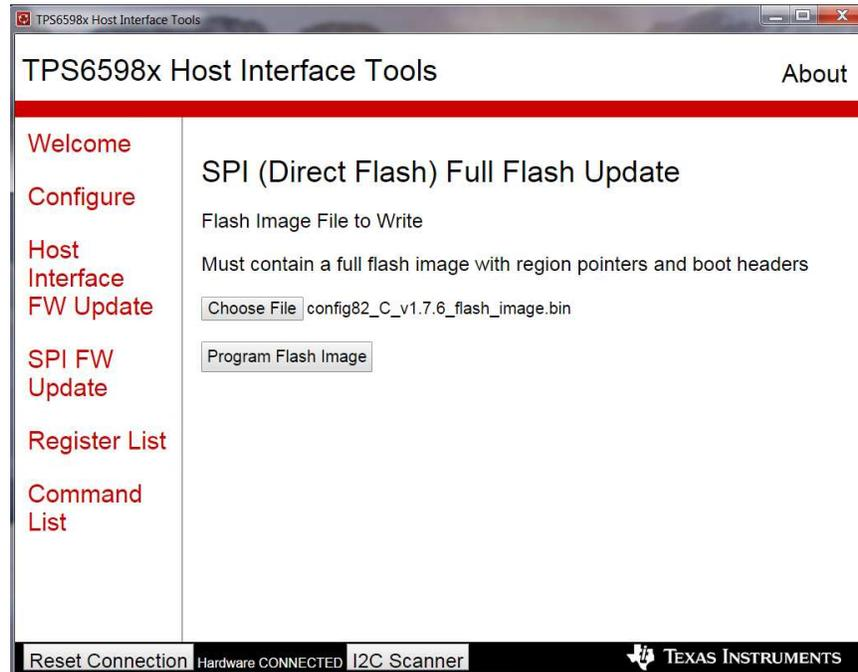
**Figure 27. SPI FW Update on TPS65982 Utilities GUI**
