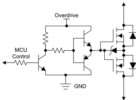
**Figure 5. Push/Pull Control Circuit with Bidirectional Switch**
