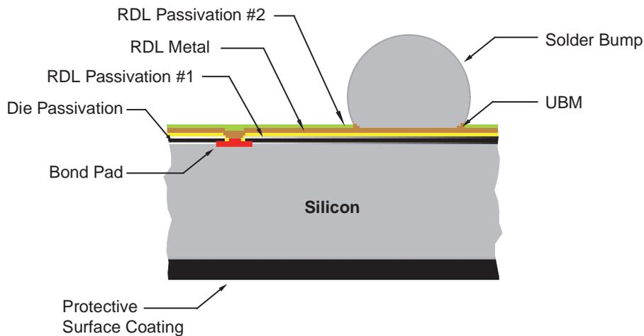
**Figure 4. RDL WCSP Construction Cross-Section**
