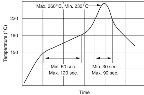
**Figure 18. Recommended Reflow Profiles**
