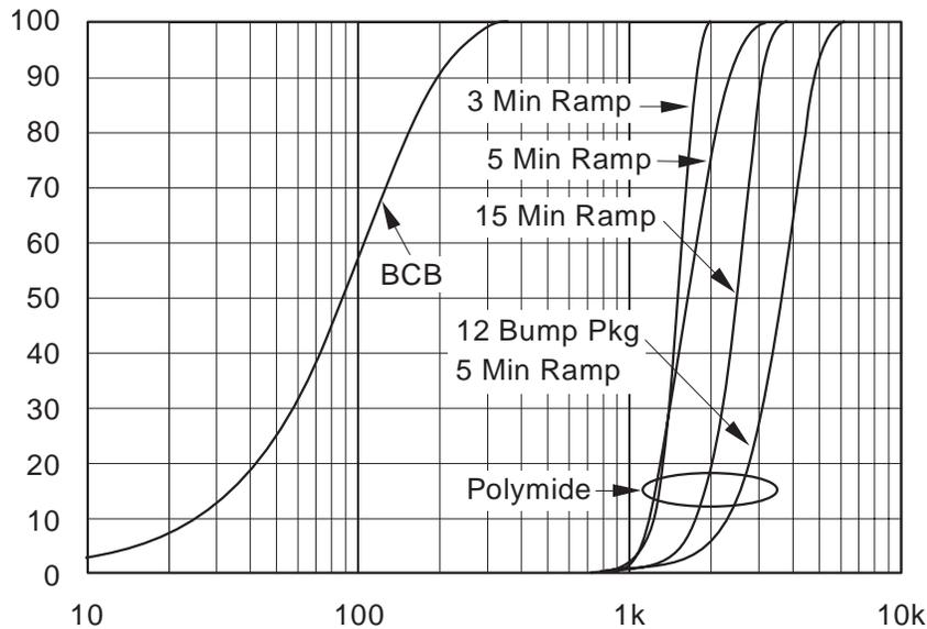
**Figure 11. N25 TCT Weibull Comparison of Ramp Rates and Materials**
