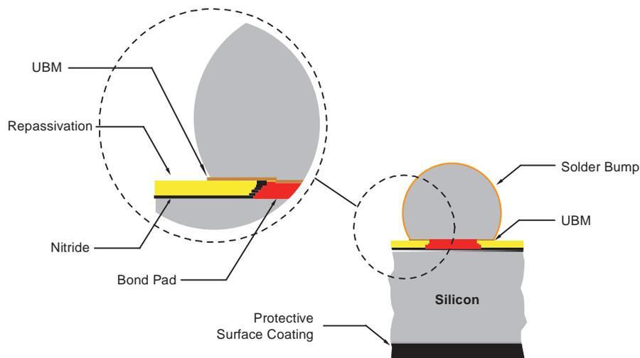
**Figure 3. Direct Bump WCSP Construction Cross-Section**
