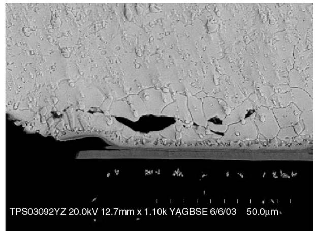
**Figure 15. Enlargement of Crack Area in Figure 14**
