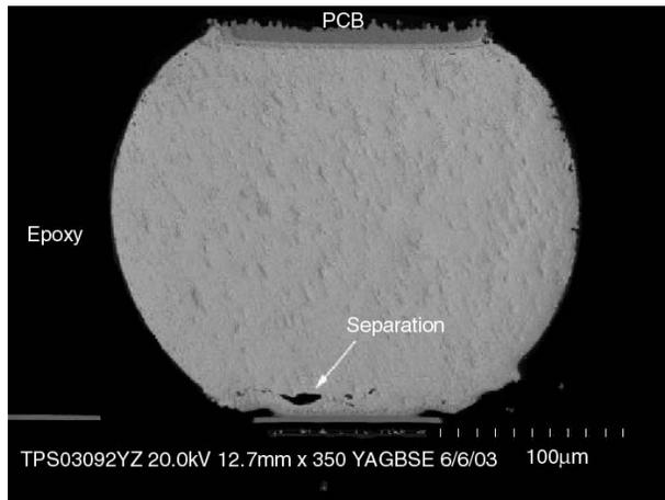
**Figure 14. Typical Lead-Free BLR Solder Fatigue Crack**
