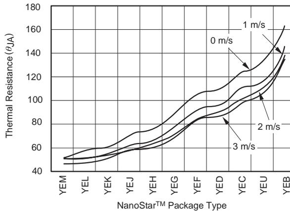
**Figure 7. JEDEC 2S2P Thermal Performance Data Graph**
