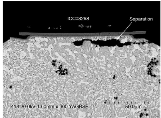
**Figure 13. Enlargement of Crack Area in Figure 12**
