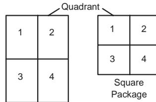
**Figure 21. Carrier-Tape Cavity Quadrant Location for Pin 1, per EIA-481B**
