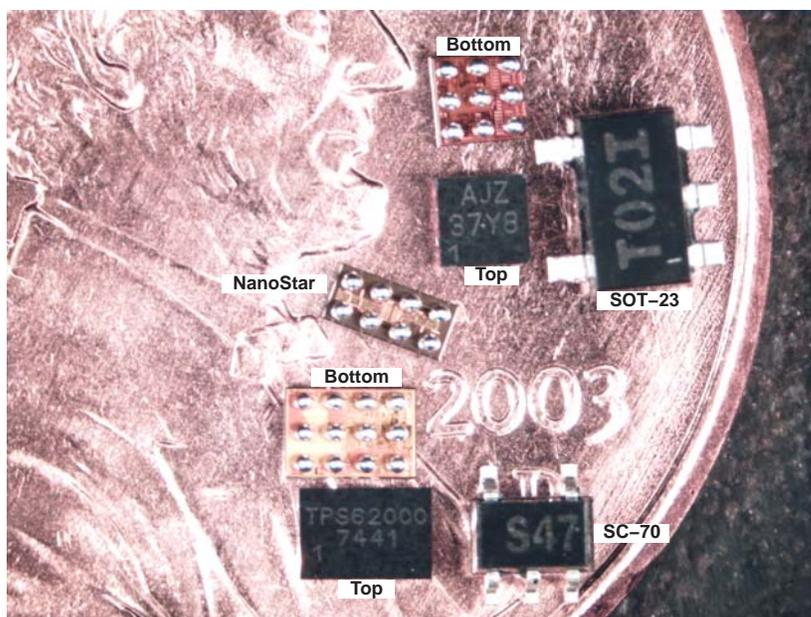
**Figure 1. NanoStar™ WCSP, SOT-23, & SC-70 Size Comparison**
