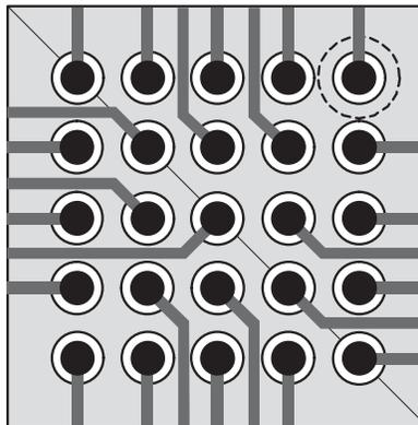
**Figure 16. Example of 5x5 Array Balanced Routing Pattern**
