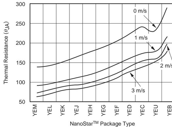
**Figure 6. JEDEC 1S0P Thermal Performance Data Graph**
