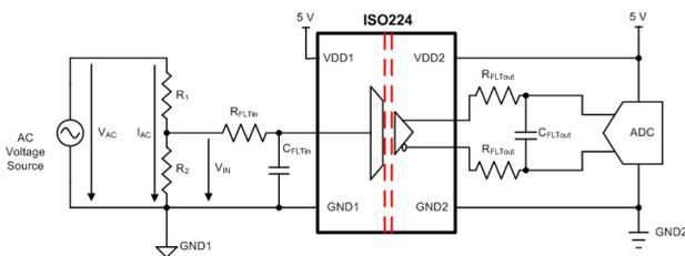
Figure 1. AC Voltage Sensing with the ISO224
