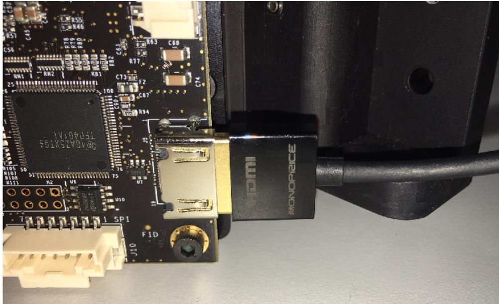
**Figure 2-4. HDMI Cable Install**
