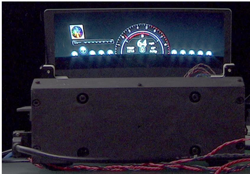
**Figure 2-9. Example of C-HUD Displaying Video Content**
