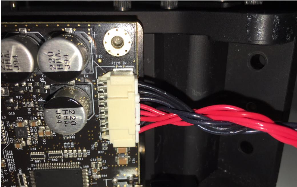
**Figure 2-5. Power Cable Install**
