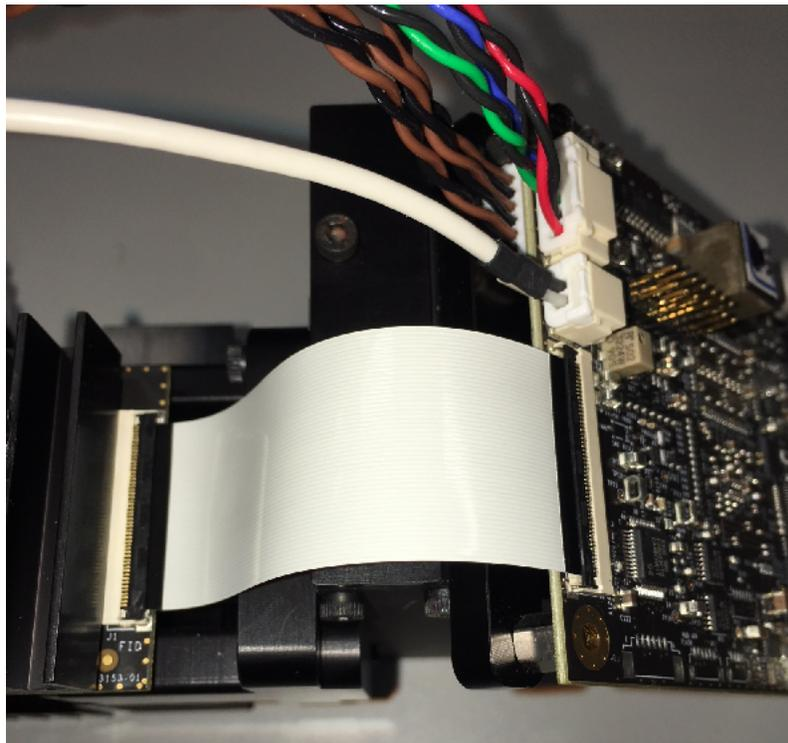
**Figure 2-2. Installation of PGU Cables into Formatter Board**
