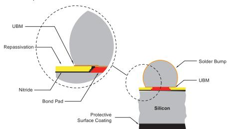
Figure 3. Direct Bump WCSP Construction Cross-Section
