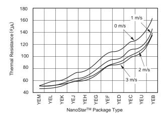
Figure 7. JEDEC 2S2P Thermal Performance Data Graph
