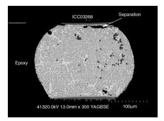
Figure 12. Typical Tin-Lead BLR Solder Fatigue Crack
