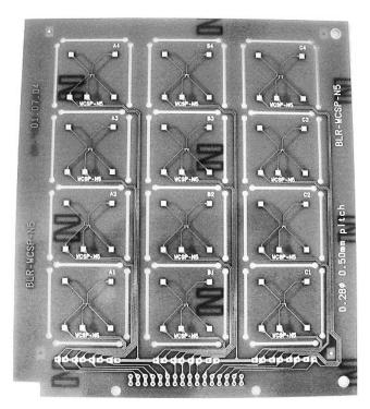
Figure 10. 12-Site Thermal Cycle Test BLR Test Board
