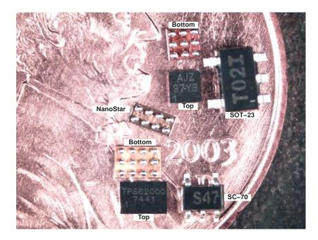
Figure 1. NanoStar<sup>™</sup> WCSP, SOT-23, & SC-70 Size Comparison
