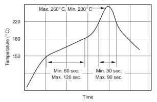
Figure 18. Recommended Reflow Profiles
