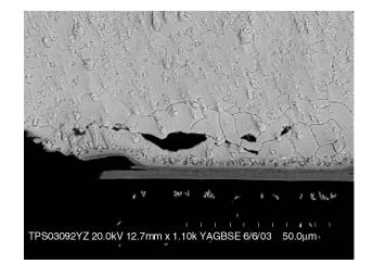
Figure 15. Enlargement of Crack Area in Figure 14
