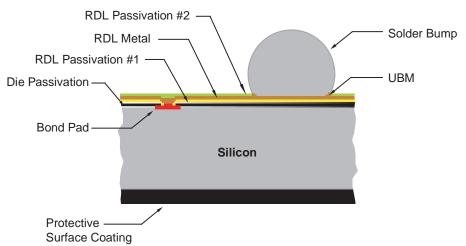
Figure 4. RDL WCSP Construction Cross-Section
