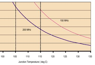
Electromigration: Life versus Junction Temperature. Maintaining the proper junction temperature prolongs device life; reducing clock speed is beneficial to both.
