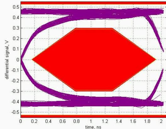
Figure 9-4. HighSpeed TX Eye for Downstream Port 2
