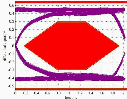
Figure 9-3. HighSpeed TX Eye for Downstream Port 1
