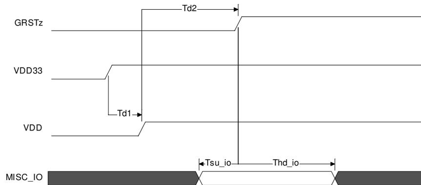
**Figure 7-1. Power-Up Timing Requirements**
