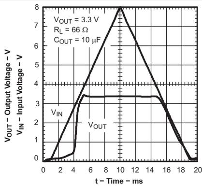
Figure 11. Power-Up and Power-Down
