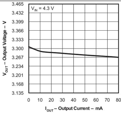
Figure 1. TPS715A33 Output Voltage vs Output Current
