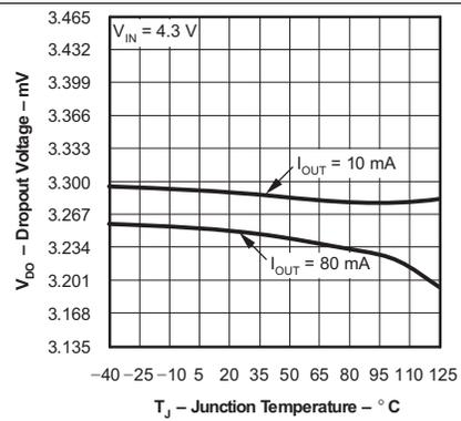
Figure 2. TPS715A33 Dropout Voltage vs Junction Temperature
