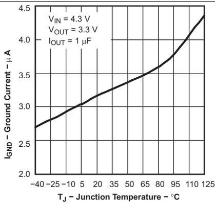
Figure 3. Ground Current vs Junction Temperature
