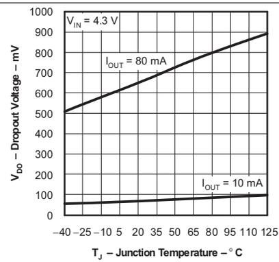
Figure 8. TPS715A33 Dropout Voltage vs Junction Temperature
