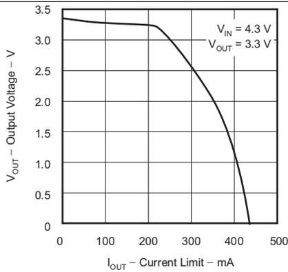
Figure 9. Output Voltage vs Current Limit
