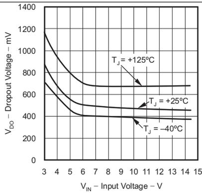
Figure 7. TPS715A01 Dropout Voltage vs Input Voltage
