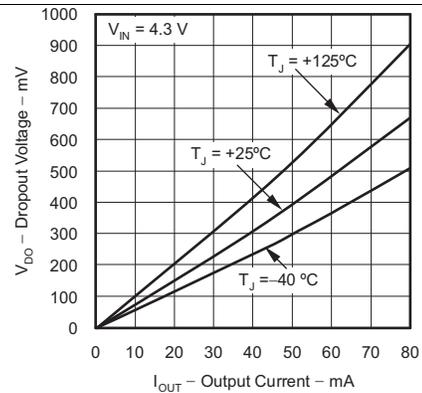
Figure 6. TPS715A33 Dropout Voltage vs Output Current
