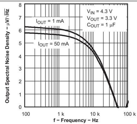
Figure 4. Output Spectral Noise Density vs Frequency
