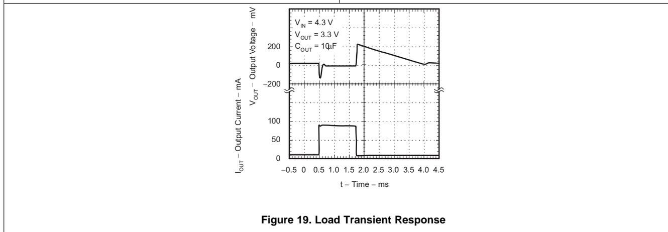
Figure 19. Load Transient Response
