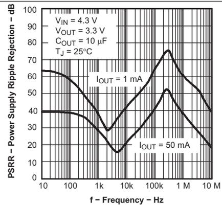
Figure 10. Power-Supply Ripple Rejection vs Frequency
