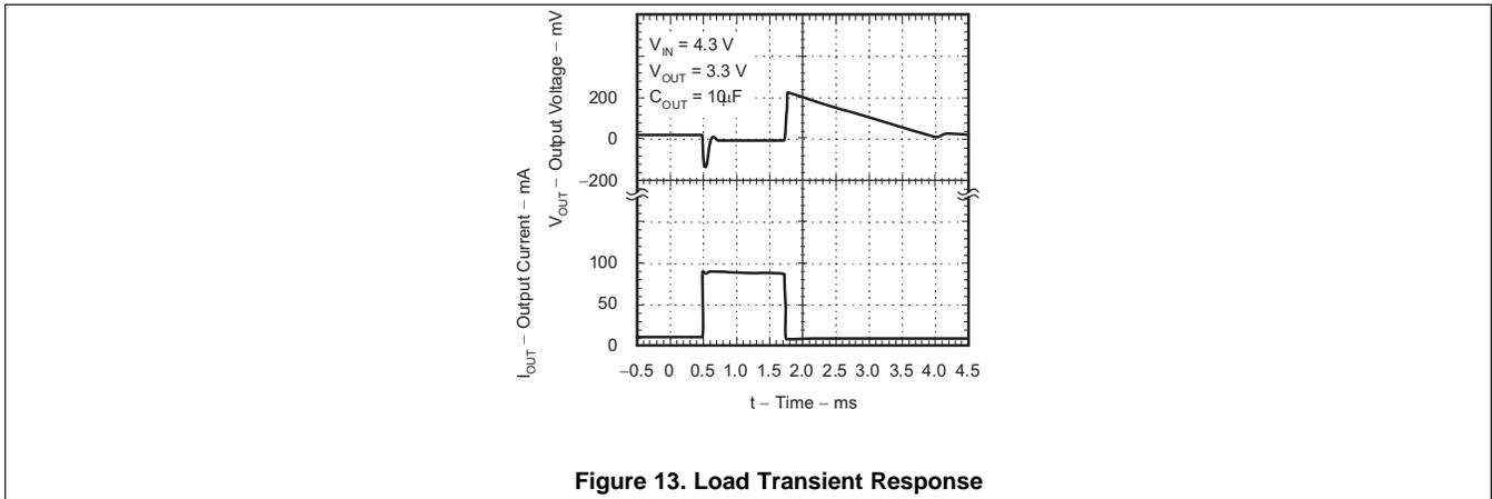
**Figure 13. Load Transient Response**
