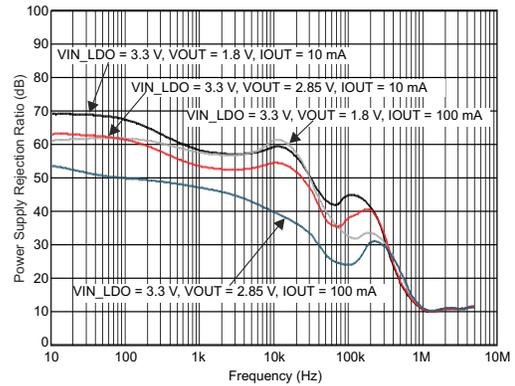
**Figure 6-26. LDO6 and LDO8 PSRR vs Frequency**
