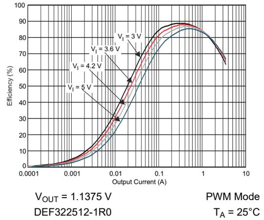
Figure 6-20. DCDC4 Efficiency vs Output Current
