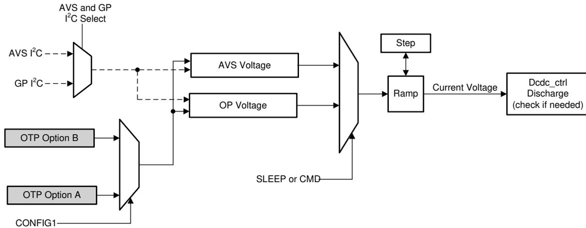
**Figure 8-11. DC-DC Voltage Scaling Architecture**
