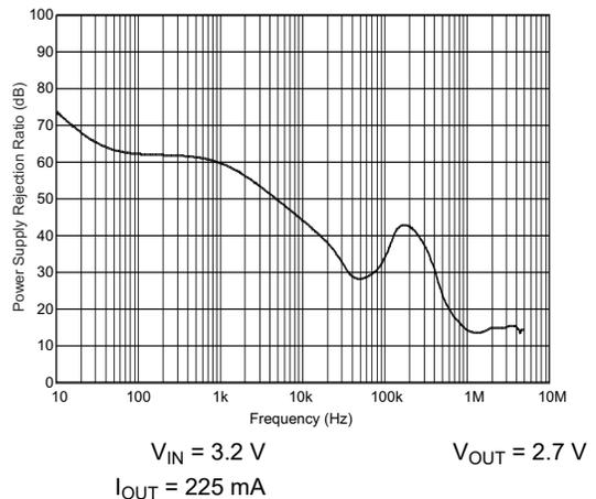
Figure 6-24. LDO4 and LDO5 PSRR vs Frequency
