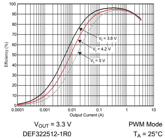
Figure 6-22. DCDC4 Efficiency vs Output Current
