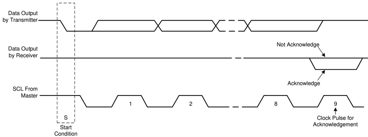
**Figure 8-21. Acknowledge on the I<sup>2</sup>C Bus**
