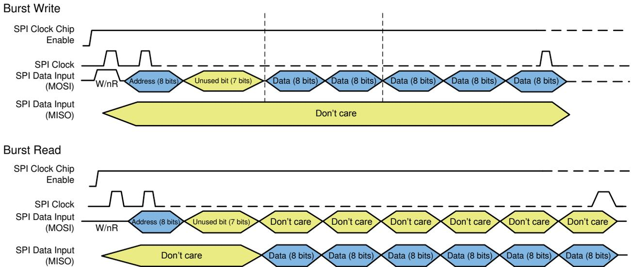
**Figure 8-18. SPI BURST READ and BURST WRITE Protocol**
