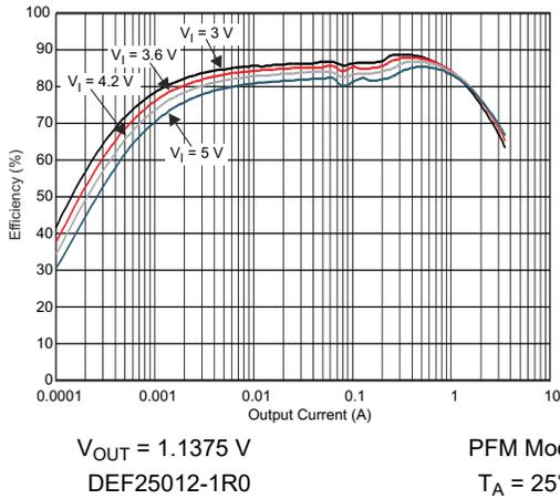
Figure 6-19. DCDC4 Efficiency vs Output Current
