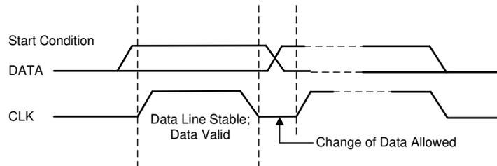
**Figure 8-20. Bit Transfer on the Serial Interface**
