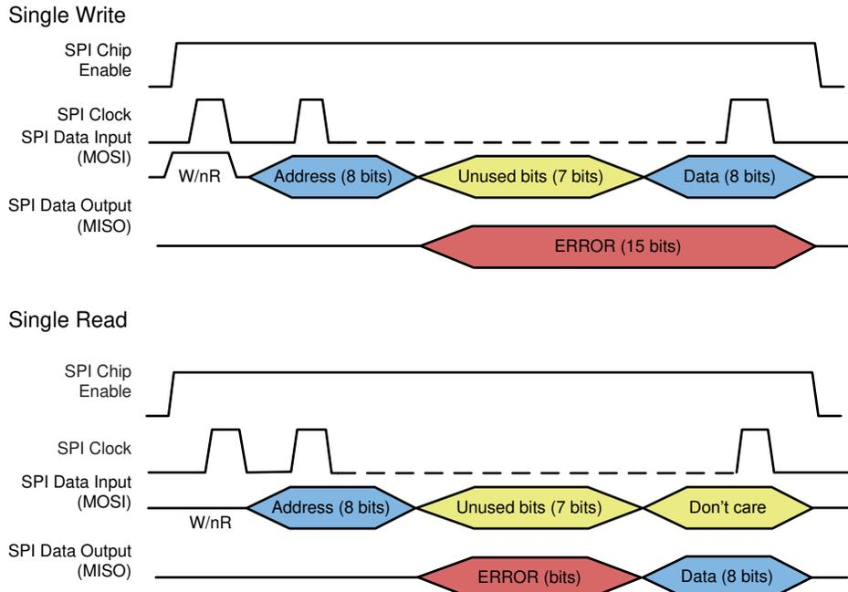
**Figure 8-17. SPI READ and WRITE Protocol**
