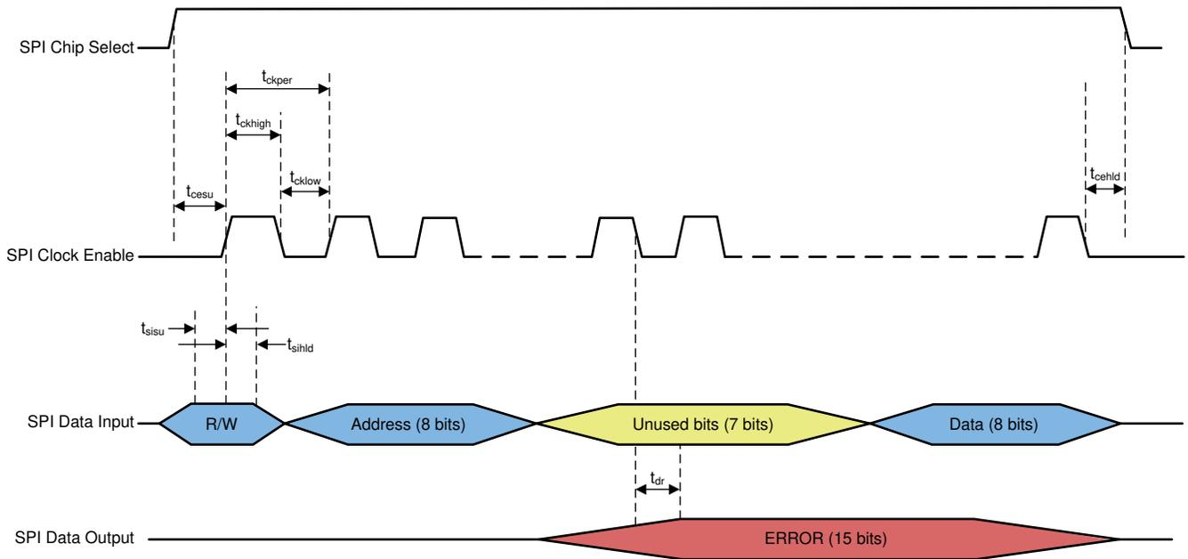
**Figure 7-3. SPI Timing**
