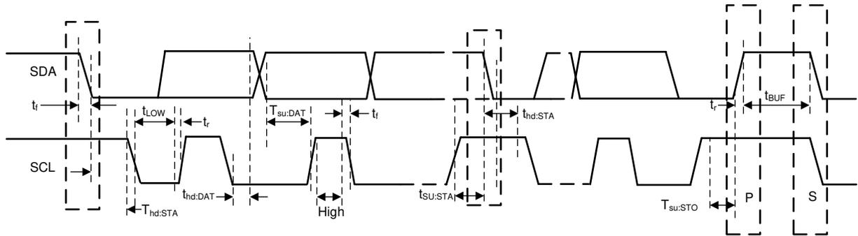
**Figure 7-1. Serial Interface Timing Diagram for FS-Mode**
