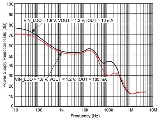
Figure 6-23. LDO1, LDO2, LDO3 PSRR vs Frequency
