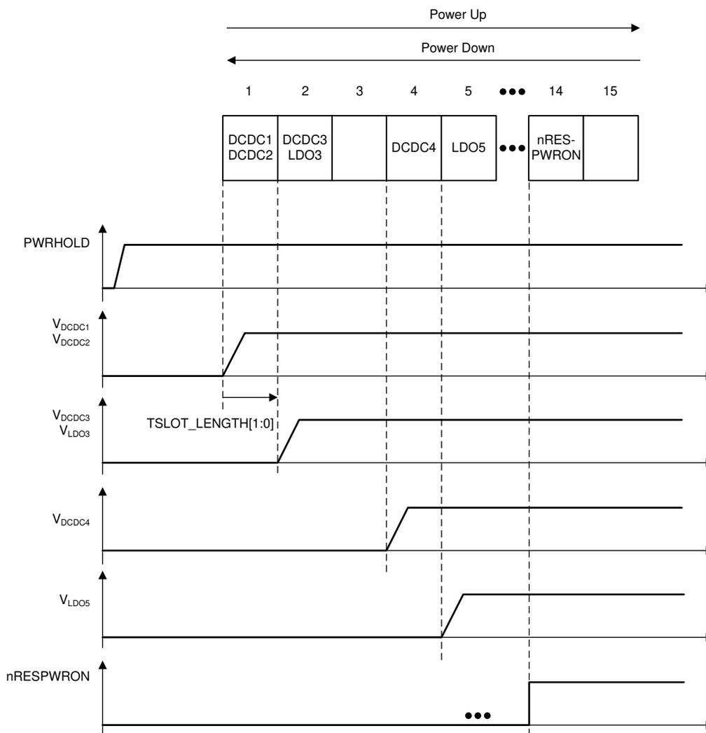
**Figure 8-9. Internal Power-Up Example**
