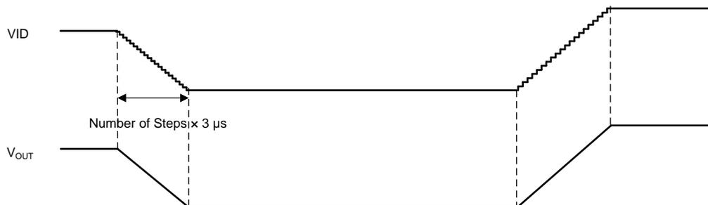
Figure 5-4. DVS Timing Diagram I (BUCKx\_DECAY = 0b)
