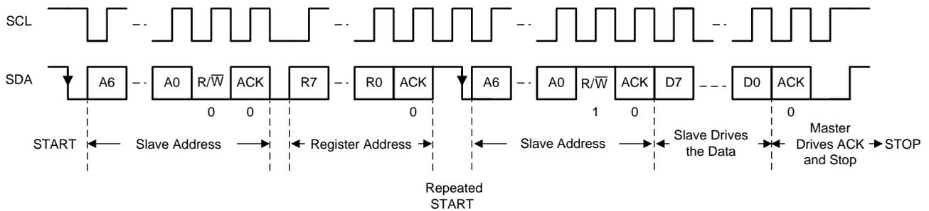
Figure 5-14. I<sup>2</sup>C Interface READ From TPS6508700 in F/S Mode (Only Repeated START is Supported)
