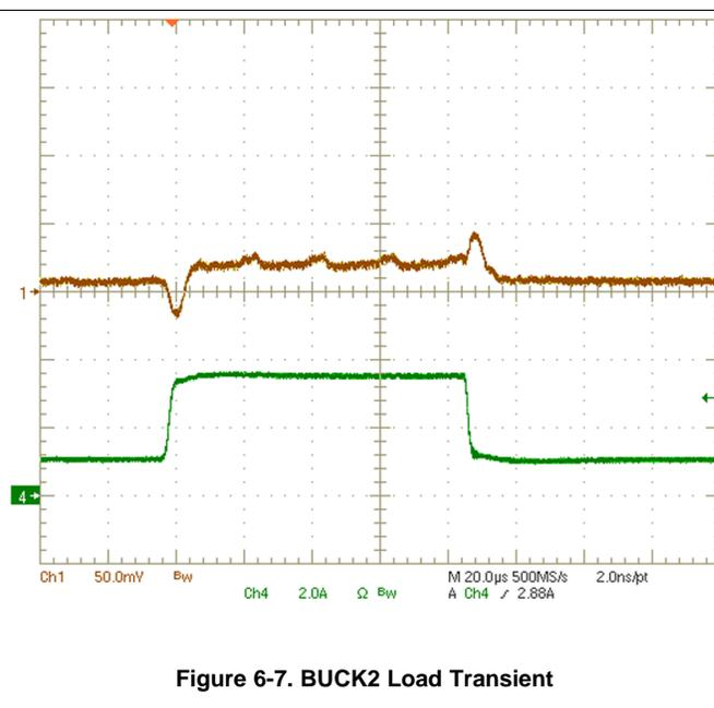
Figure 6-7. BUCK2 Load Transient
