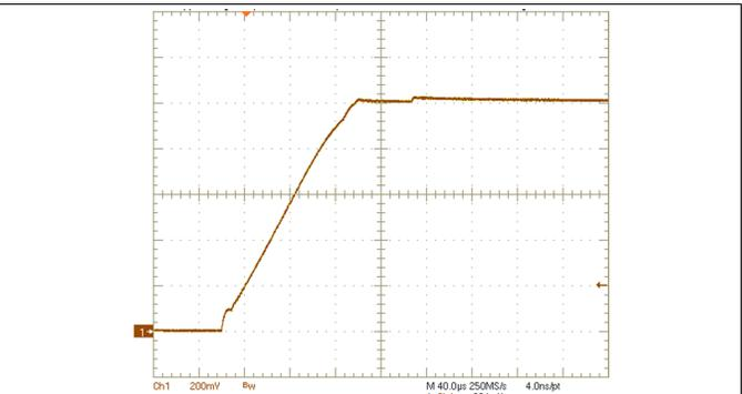
Figure 4-2. Converter Start Up to 1 V by I<sup>2</sup>C
