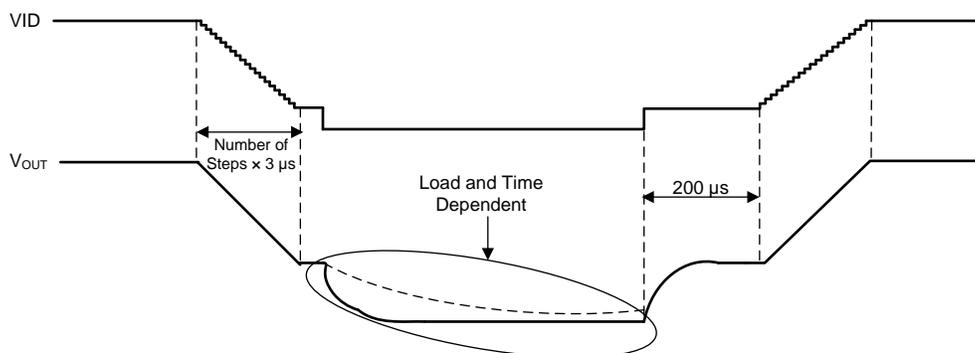
Figure 5-5. DVS Timing Diagram II (BUCKx\_DECAY = 0b)
