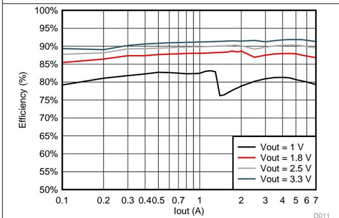
Figure 4-3. BUCK6 Efficiency at  $V_{IN} = 13\text{ V}$
