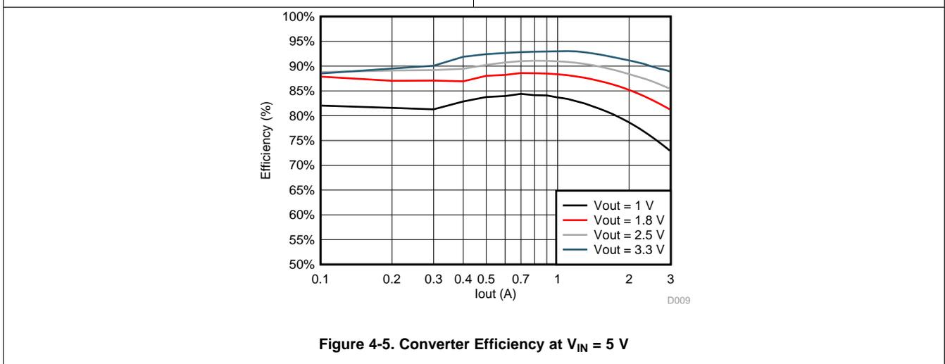
Figure 4-5. Converter Efficiency at  $V_{IN} = 5\text{ V}$
