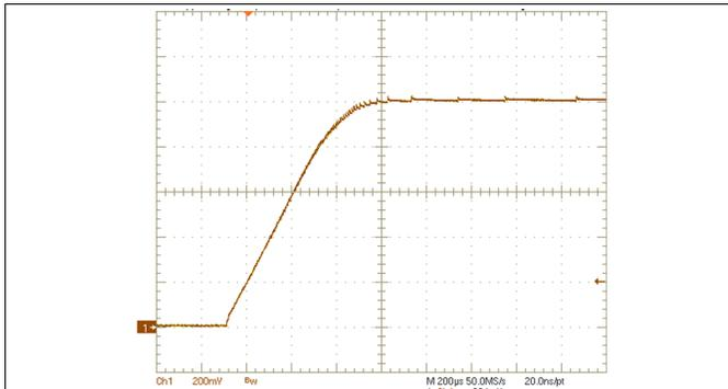
Figure 4-1. BUCK2 Controller Start Up to 1 V by I<sup>2</sup>C
