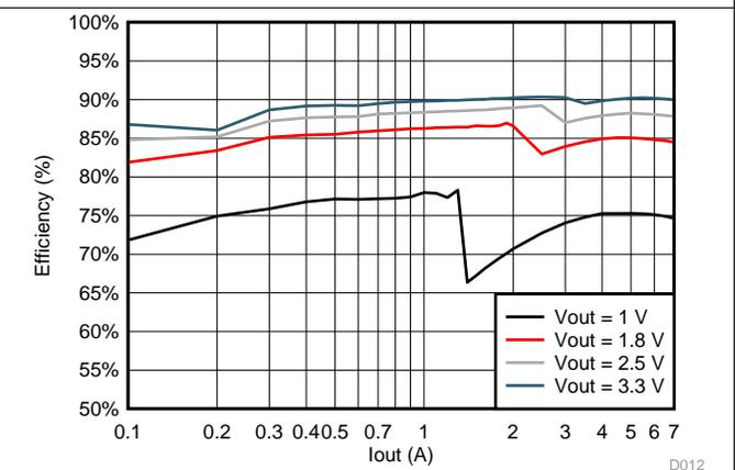
Figure 4-4. BUCK6 Efficiency at  $V_{IN} = 18\text{ V}$
