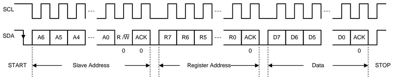
Figure 5-13. I<sup>2</sup>C Interface WRITE to TPS6508700 in F/S Mode
