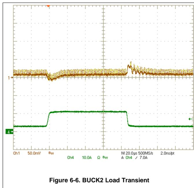
Figure 6-6. BUCK2 Load Transient
