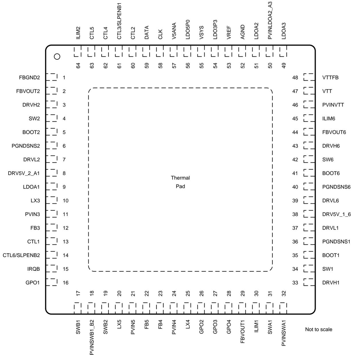
The thermal pad must be connected to the system power ground plane.
