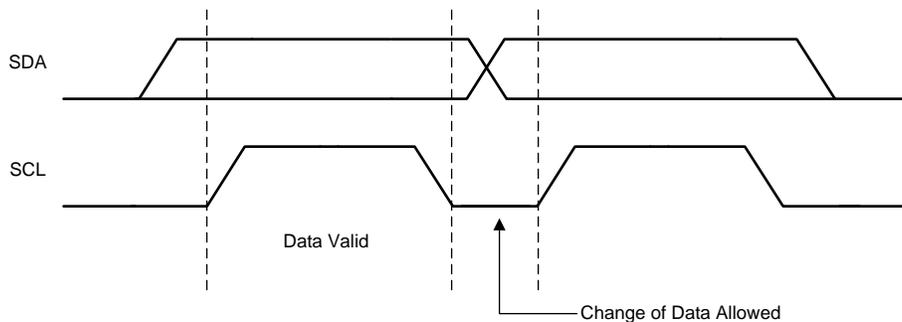
Figure 5-10. Bit Transfer on the I<sup>2</sup>C Bus
