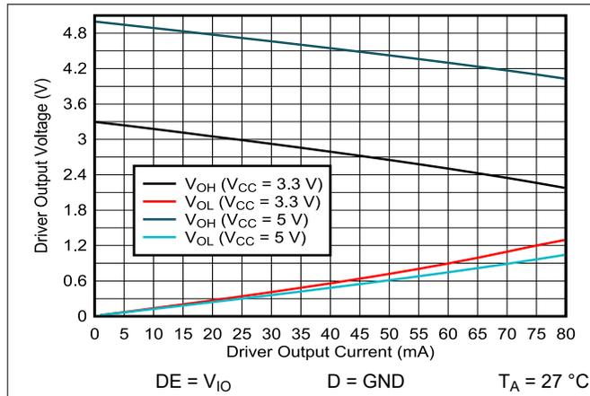
**Figure 5-1. Driver Output Voltage vs Driver Output Current**
