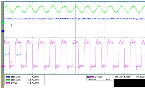
A pin given  $\pm 200\text{mV } V_{ID}$  with DC offset of 1.5 V
