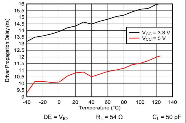
**Figure 5-10. THVD2450V 20Mbps Driver propagation delay vs Temperature**
