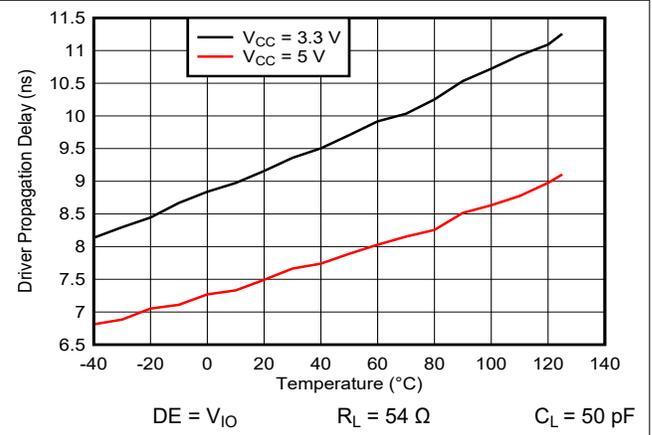
**Figure 5-12. THVD2450V 50Mbps Driver propagation delay vs Temperature**
