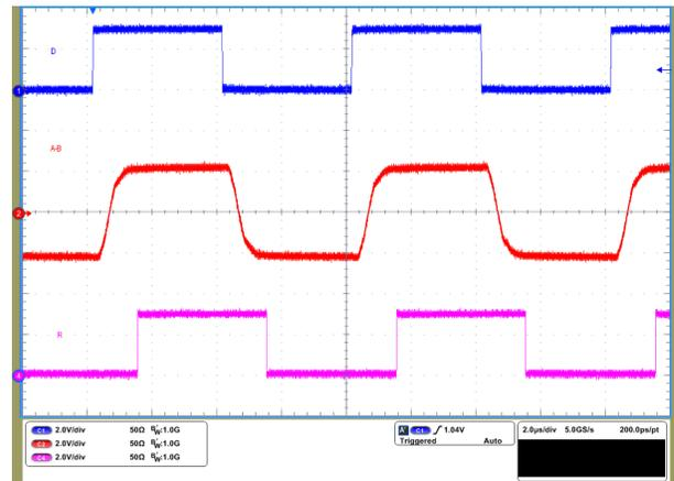
50% duty square wave on D pin at 250 kbps
