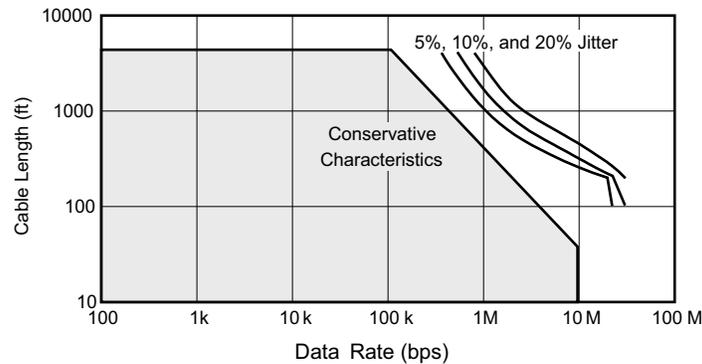
**Figure 8-3. Cable Length vs Data Rate Characteristic**
