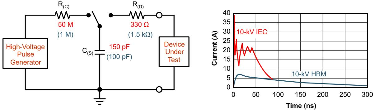
Figure 8-4. HBM and IEC ESD Models and Currents in Comparison (HBM Values in Parenthesis)
