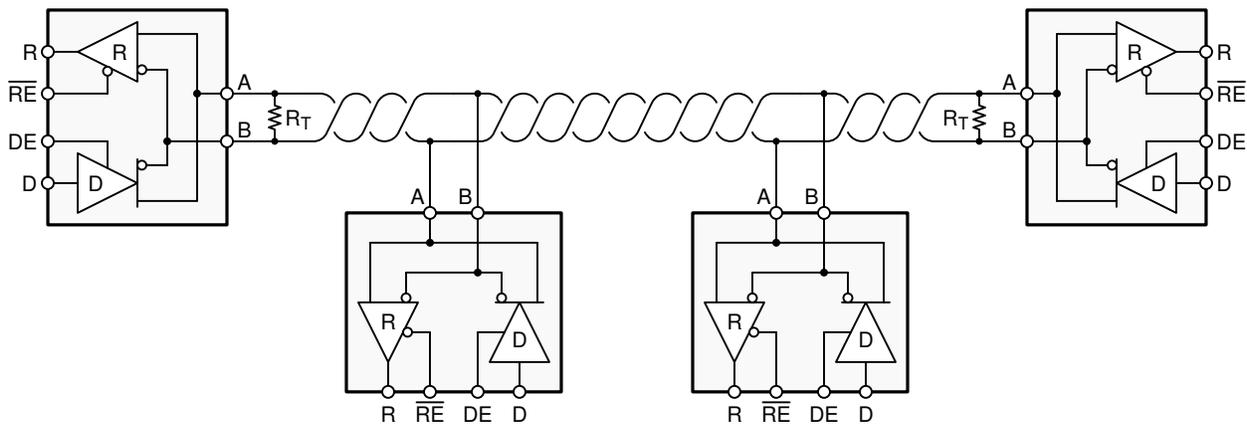
**Figure 8-1. Typical RS-485 Network With Half-Duplex Transceivers**
