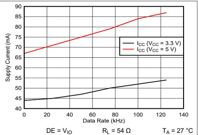
Figure 5-14. THVD2410V Supply Current vs Signal Rate
