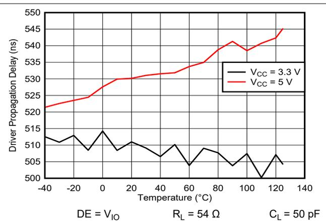
**Figure 5-6. THVD2410V 250kbps Driver propagation delay vs Temperature**
