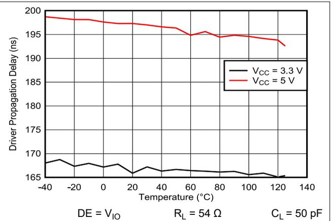
**Figure 5-8. THVD2410V 1Mbps Driver propagation delay vs Temperature**
