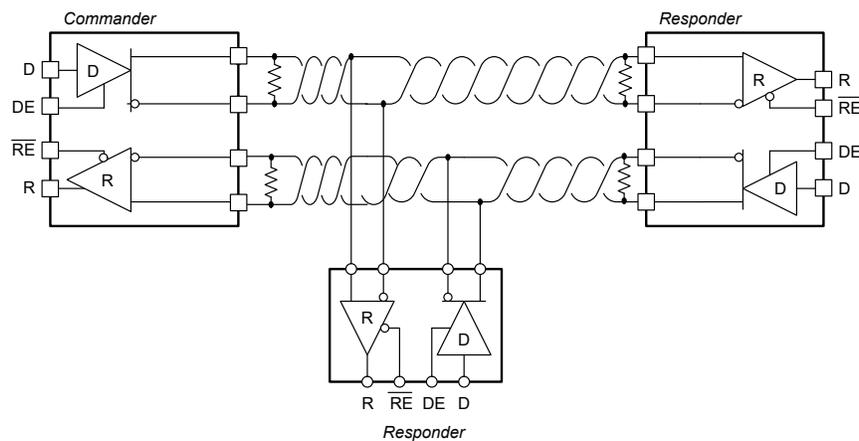
**Figure 8-2. Typical RS-485 Network with Full-Duplex transceivers**
