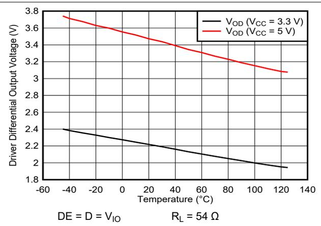
**Figure 5-4. Driver differential output voltage vs Temperature**
