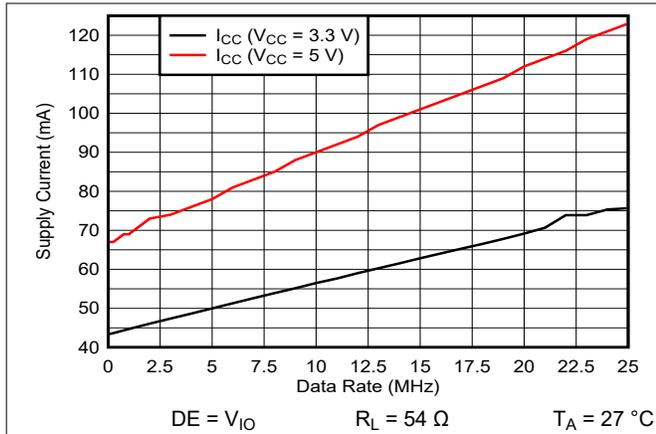
Figure 5-13. THVD2450V Supply Current vs Signal Rate
