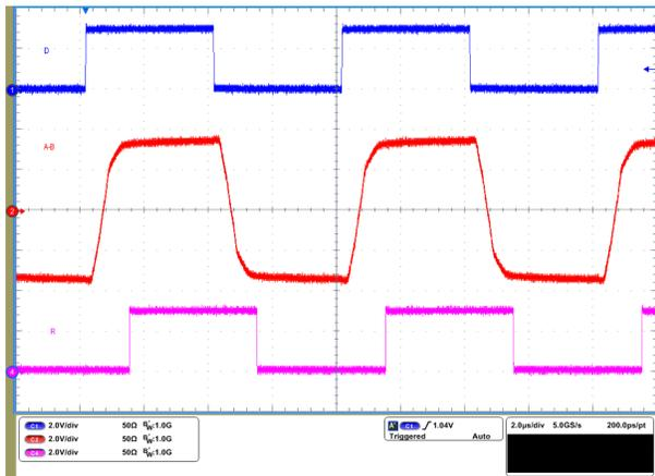
50% duty square wave on D pin at 250 kbps
