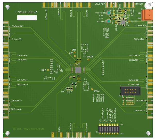
Figure 11-1. LMK00334-Q1 Layout Example
