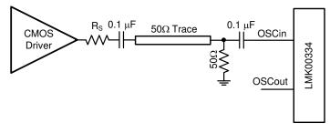
Figure 9-4. Driving OSCin With a Single-Ended Input
