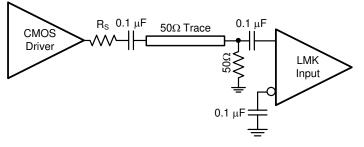
Figure 9-2. Single-Ended LVCMOS Input, AC Coupling
