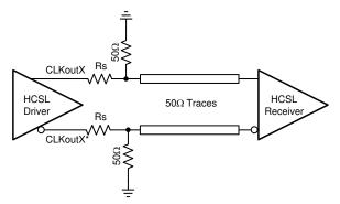
Figure 9-6. HCSL Operation, DC Coupling
