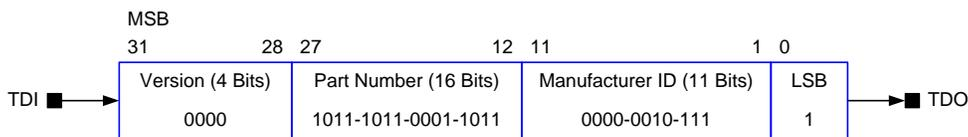
Figure 14. DMD Device ID and 32-bit Shift Order
