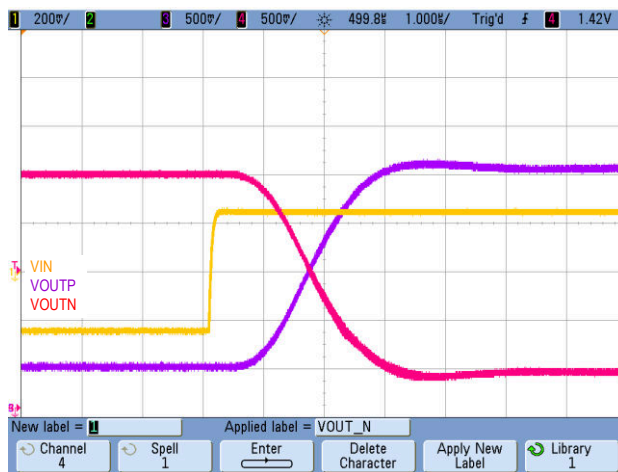
Figure 8-4. Step Response of the AMC1301
