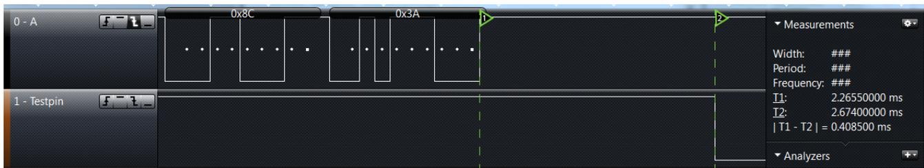
**Figure 9. Logic Analyzer Plot of Data Transfer at 38400 bps With Long Timeout**
