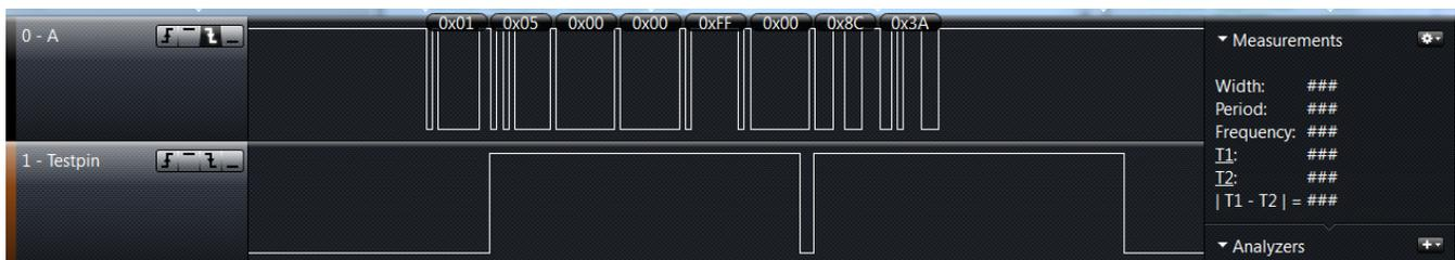
**Figure 10. Logic Analyzer Plot of Data Transfer at 38400 bps With Short Timeout**
