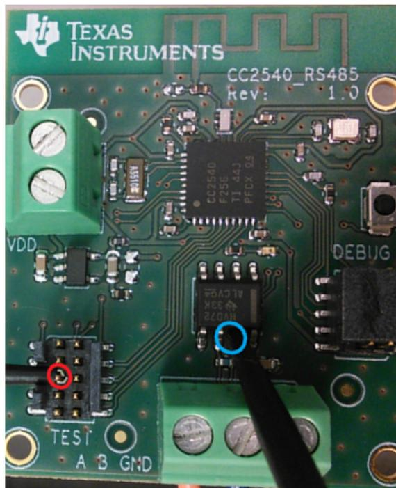
**Figure 11. Logic Analyzer Connected to P0\_6 (Red) and Either A or B (Blue)**
