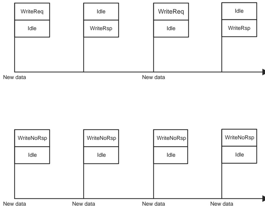
**Figure 6. Transmitting Using Regular Write Command versus No Response Command**
