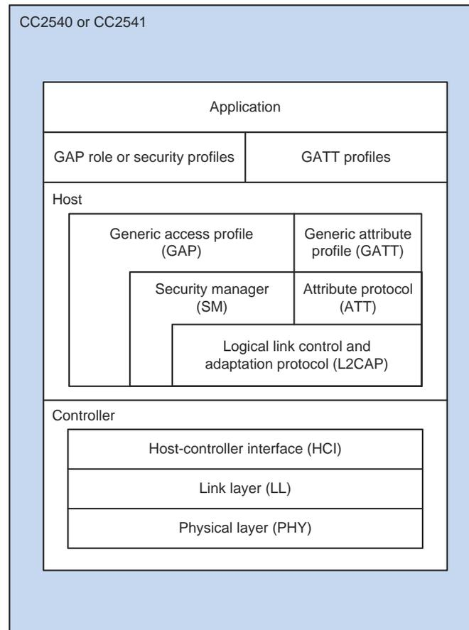
**Figure 5. Software Architecture of BLE Device**
