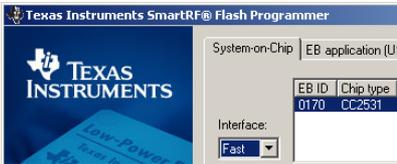
The Flash Programmer application, available on the kit web page [3], can be used to program Intel HEX files, read the contents of flash and several other operations.
