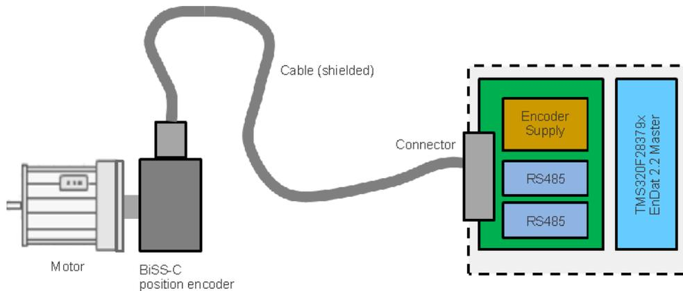
**Figure 1-1. Industrial Servo Drive With BiSS-C Position Encoder Interface**
