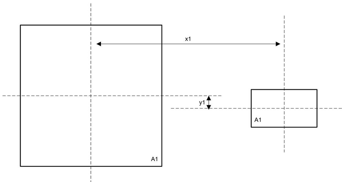
**Figure 3-2. LPDDR4 Placement Specification**
