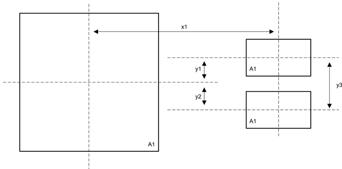
**Figure 2-3. DDR4 Placement Specifications**
