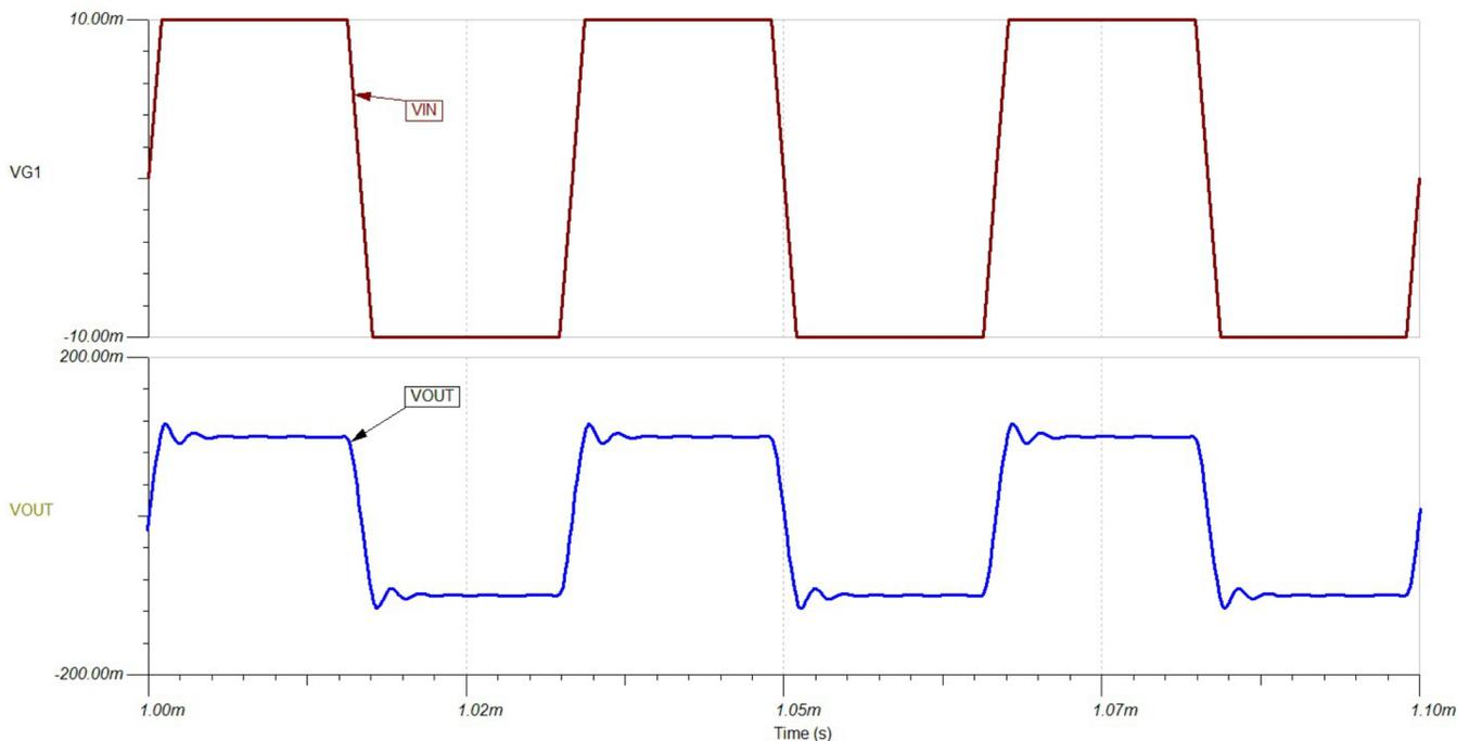
**Figure 11. Transient Response - Active Feedback with Secondary Compensation**
