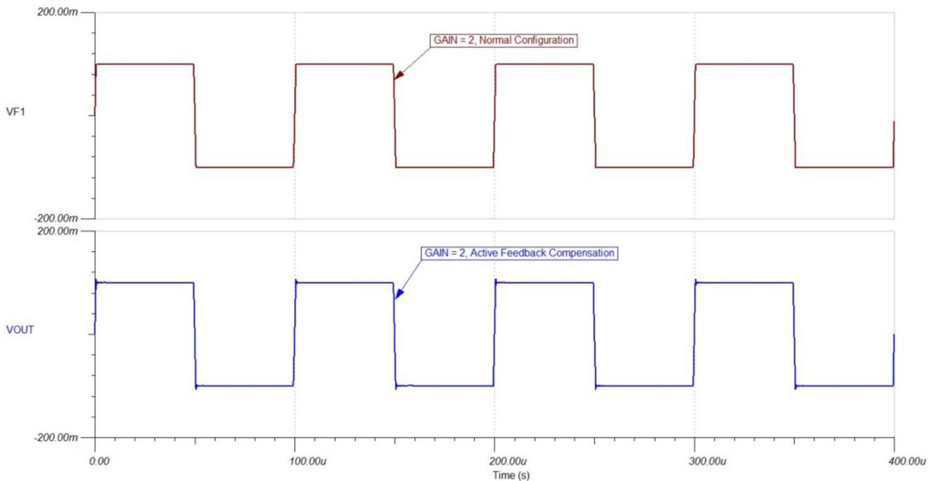
Figure 8. Transient Response of the System with Gain 2
