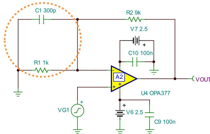
Figure 1. Phase Compensation Using RC Circuit
