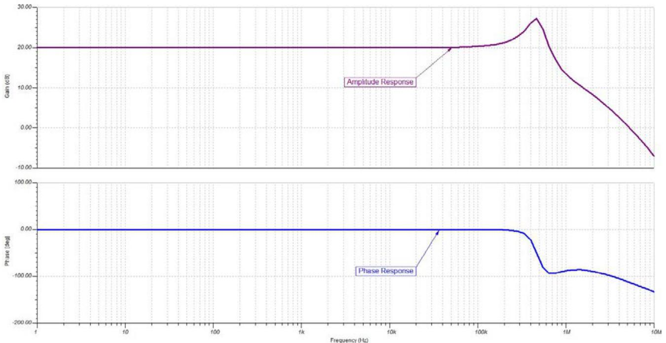
Figure 10. Amplitude and Phase Response of Secondary Compensation
