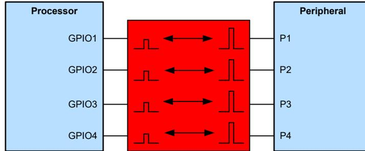
**Example GPIO Voltage Translation Block Diagram**
