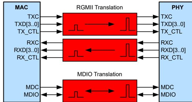
Figure 7-1. Example MAC to PHY Voltage Translation Block Diagram
