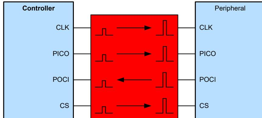
**Example SPI Voltage Translation Block Diagram**
