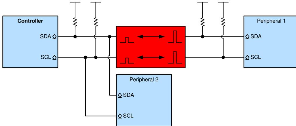
Example of Using Voltage Translation With an I<sup>2</sup>C Communication Bus
