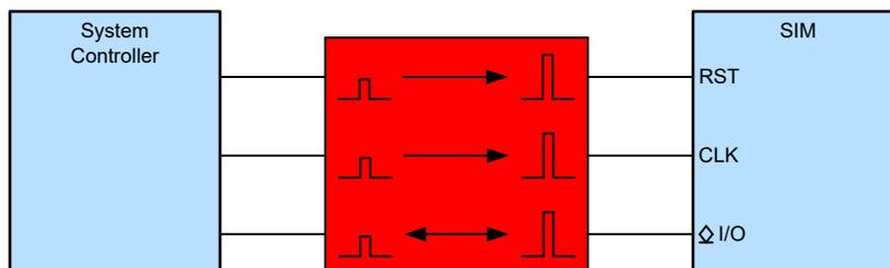
Figure 8-1. Example SIM Card Voltage Translation Block Diagram
