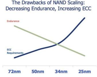
Figure 2: Device issues versus process node shrinks (courtesy Micron)
