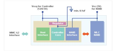
Figure 3. eMMC block diagram (courtesy Samsung)
