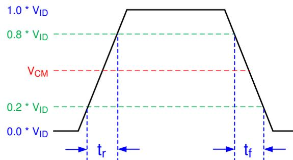
Figure 3. SubLVDS Input Rise and Fall Slew Rate
