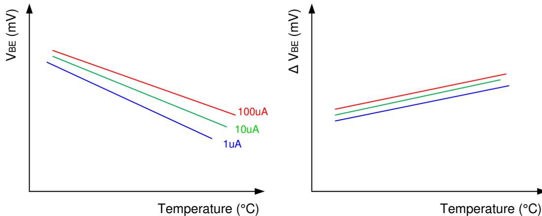
**Figure 18. Example of Delta VBE Versus Temperature**
