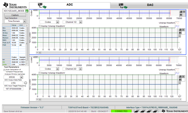
图 8-10. Idle-Channel Noise (No Input) for 2.5-GSPS, Dual-Channel Oscilloscope
