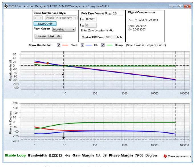
图 36. Voltage Loop Design Using Compensation Designer
