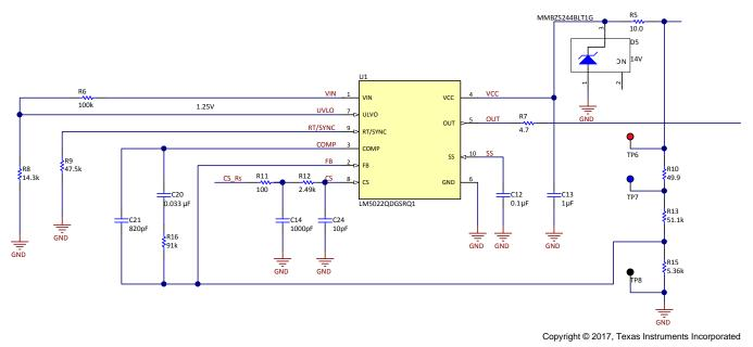
Figure 6. Compensation Network of Flyback DC-DC Converter
