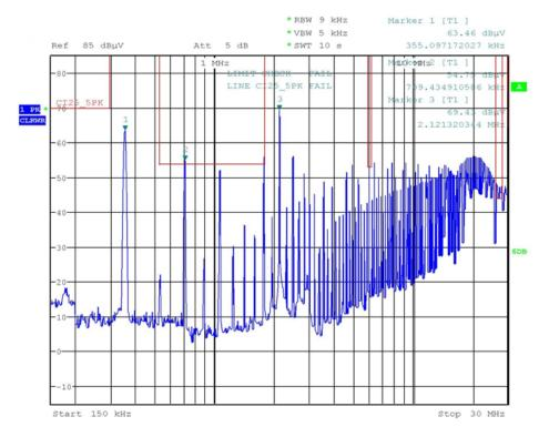
Figure 36. Peak Noise of TIDA-01344 With  $V_{IN}$  = 10 V and  $I_{OUT}$  = 1.7 A
