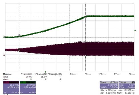
Figure 13. Start-up Waveform of Flyback Converter With  $V_{IN}$  = 11 V,  $I_{OUT}$  = 1.3 A
