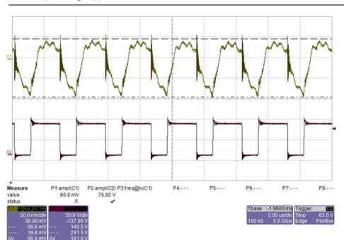
**NOTE:** CH1: Output voltage ripple, CH2: Switch node
