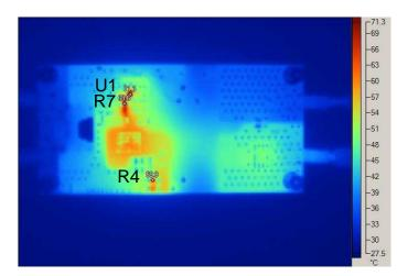
Figure 27. Thermal Image of TIDA-01344 With V<sub>IN</sub> = 48 V and P<sub>OUT</sub> = 23.8 W (PCB Bottom Side)
