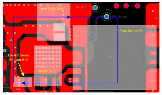
Figure 57. Current Flow Loop in Power Stage
