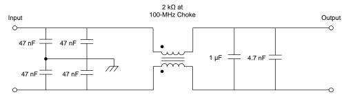
Figure 42. Implemented External CM Filter
