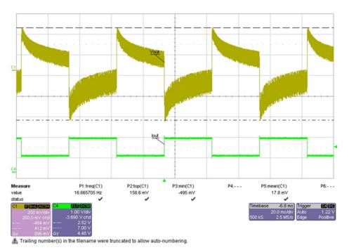
Figure 24. Load Transient Response Under  $V_{IN}$  = 48 V and  $I_{OUT}$  Switching Between 0.8 A and 1.7 A
