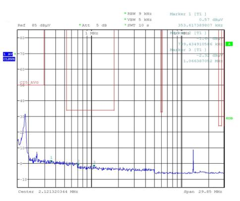
Figure 34. Ambient Noise (Average Measurement: 150 kHz to 30 MHz)
