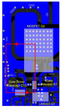
Figure 58. Gate Driver Current-Flowing Loop
