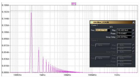
Figure 9. Fourier Component of Primary-Side Current
