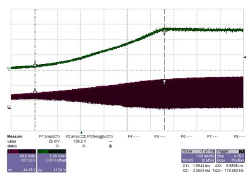
Figure 14. Start-up Waveform of Flyback Converter With V<sub>IN</sub> = 80 V, I<sub>OUT</sub> = 1.3 A
