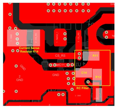
Figure 60. Placement of the RC Filtering Network for LM5022-Q1 Current Sense Pin (Top-Side PCB)
