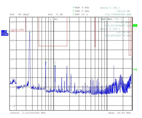
Figure 43. Peak Noise of TIDA-01344 With External Filter Under Conditions: V<sub>IN</sub> = 10 V and I<sub>OUT</sub> = 1.7 A
