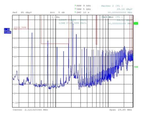
Figure 40. Peak Noise of TIDA-01344 With V\_{IN} = 80 V and I\_{OUT} = 1.7 A
