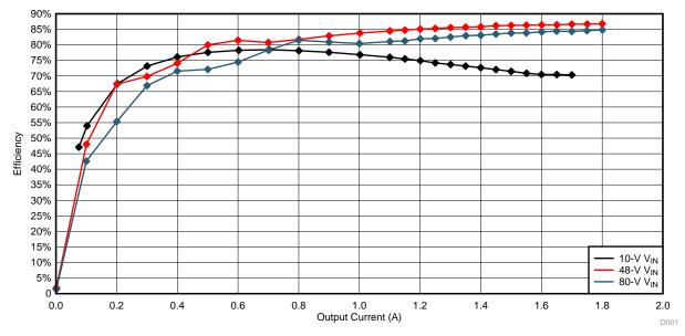
Figure 19. Measured Efficiency of TIDA-01344 Under Input Voltages of: 10 V, 48 V, and 80 V
