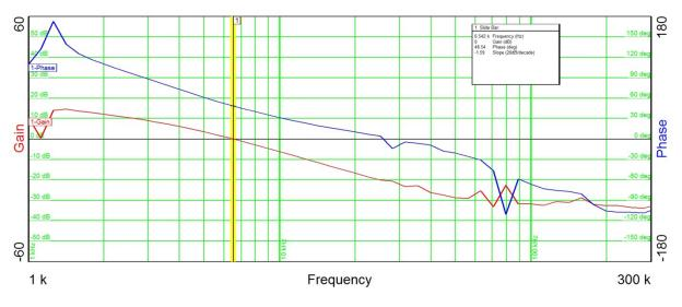
Figure 29. Loop Frequency Response of TIDA-01344 With  $V_{IN}$  = 10 V and  $I_{OUT}$  = 1.7 A
