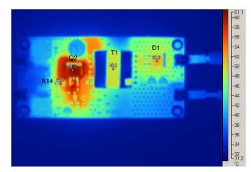
Figure 26. Thermal Image of TIDA-01344 With  $V_{IN}$  = 48 V and  $P_{OUT}$  = 23.8 W (PCB Top Side)
