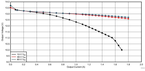
Figure 20. Load Regulation of TIDA-01344
