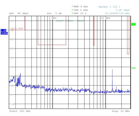
Figure 32. Ambient Noise (Peak Measurement: 150 kHz to 30 MHz)
