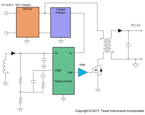
Figure 2. TIDA-01344 Block diagram
