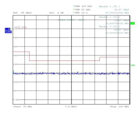
Figure 33. Ambient Noise (Peak Measurement: 30 MHz to 108 MHz)
