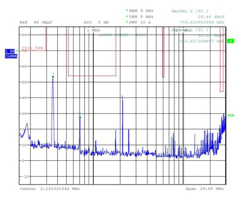
Figure 51. Peak Noise of TIDA-01344 With External Filter Under Conditions: V<sub>IN</sub> = 80 V and I<sub>OUT</sub> = 1.7 A
