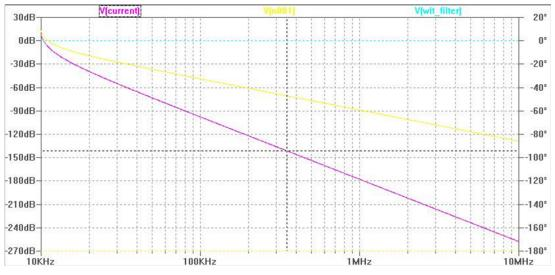
Figure 10. Simulated Frequency Response of Implemented Filter
