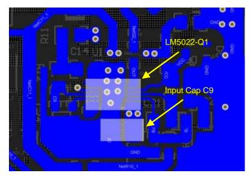
Figure 56. Placement of Input Capacitors of LM5022-Q1
