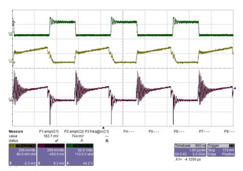
Figure 17. Comparison of Waveforms Across Current Sense Resistor and at LM5022-Q1 CS Pin
