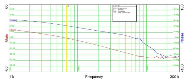
Figure 31. Loop Frequency Response of TIDA-01344 With  $V_{IN}$  = 80 V and  $I_{OUT}$  = 1.7 A
