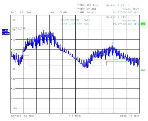
Figure 41. Peak Noise of TIDA-01344 With  $V_{IN}$  = 80 V and  $I_{OUT}$  = 1.7 A
