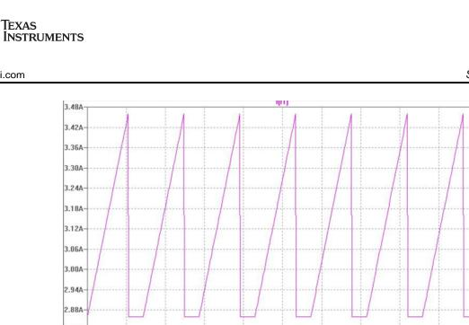
Figure 8. Triangular Current at Primary Side of Flyback
