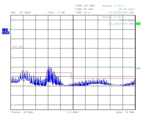
Figure 54. Average Noise of TIDA-01344 With External Filter Under Conditions: V<sub>IN</sub> = 80 V and I<sub>OUT</sub> = 1.7 A
