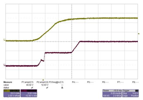
Figure 16. Start-up Waveform of LM5022-Q1 Bias Supply
