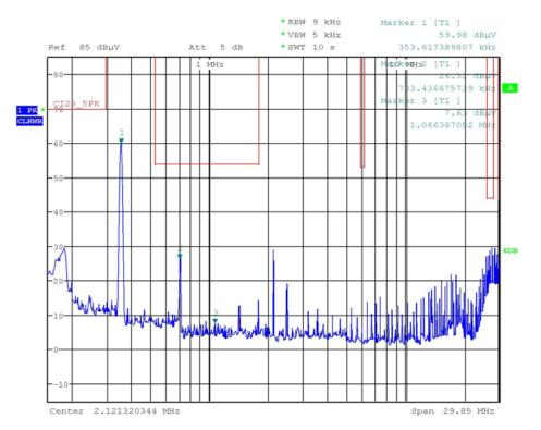
Figure 47. Peak Noise of TIDA-01344 With External Filter Under Conditions: V<sub>IN</sub> = 48 V and I<sub>OUT</sub> = 1.7 A
