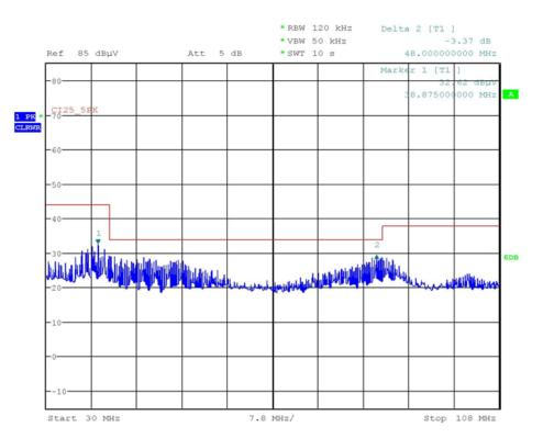
Figure 48. Peak Noise of TIDA-01344 With External Filter Under Conditions: V<sub>IN</sub> = 48 V and I<sub>OUT</sub> = 1.7 A
