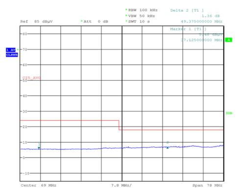
Figure 35. Ambient Noise (Average Measurement: 30 MHz to 108 MHz)
