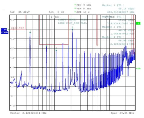
Figure 38. Peak Noise of TIDA-01344 With V<sub>IN</sub> = 48 V and I<sub>OUT</sub> = 1.7 A
