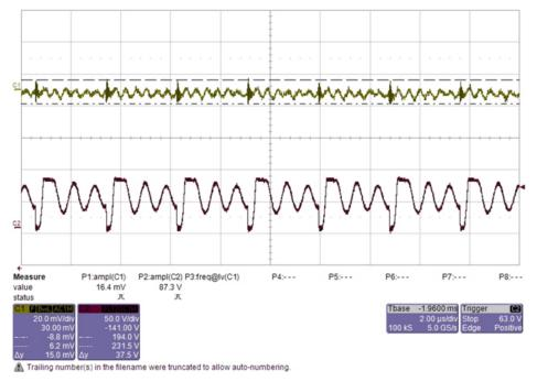
Figure 21. Output Voltage Ripple of Flyback Converter Under  $V_{IN}$  = 48 V and  $I_{OUT}$  = 0.1 A
