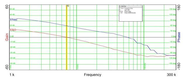
Figure 30. Loop Frequency Response of TIDA-01344 With  $V_{IN}$  = 48 V and  $I_{OUT}$  = 1.7 A
