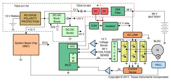
Figure 1. System Block Diagram for 48-V Battery-Driven Inverter and Implementation of TIDA-01344
