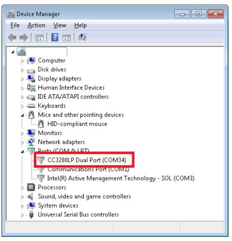
Figure 11. CC3200 COM Port in Device Manager
