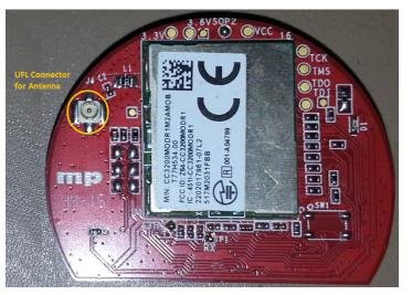
Figure 1. CC3200-MODULE UFL Connector Location
