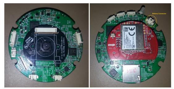
Figure 12. Assembled CC3200-MODULE and OV788 System
