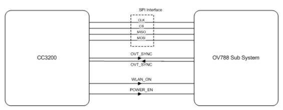
Figure 3. Diagram of Connections Between CC3200 and OV788 Subsystems
