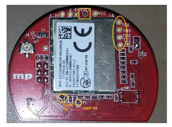
Figure 2. CC3200-MODULE Programming Interface
