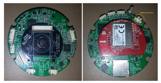
Figure 8. CC3200-MODULE Board Mounted on OV788 Subsystem
