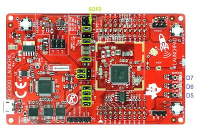
Figure 9. CC3200-LAUNCHXL Default Jumper Connections
