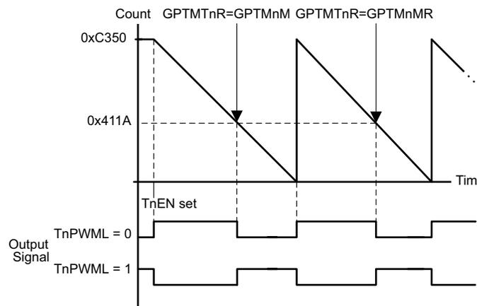
When synchronizing the timers using the GPT:SYNC register, the timer must be properly configured to avoid glitches on the CCP outputs. Both the TnPLO and the TnMRSU bits must be set in the GPT:TnMR register. Figure 13-5 shows how the CCP output operates when the TnPLO and TnMRSU bits are set and the GPT:TnMATCHR register value is greater than the GPT:TnILR register value.
