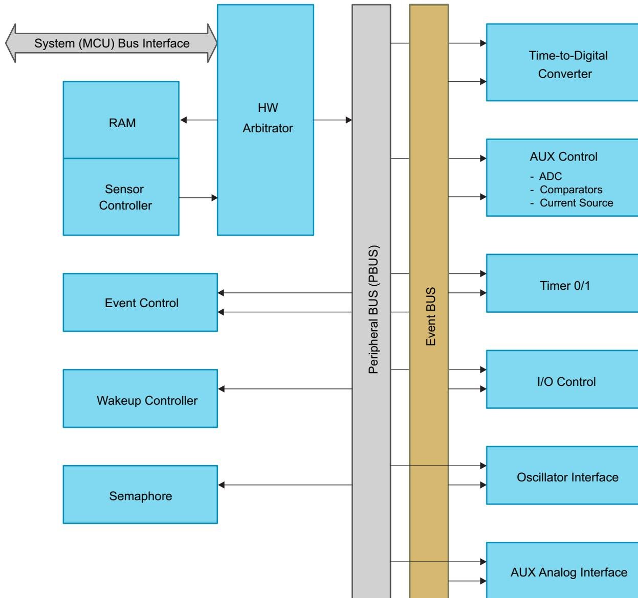
The AUX power domain is connected to the MCU system through an asynchronous interface, ensuring that all modules connected to the AUX bus are accessible from the system CPU.
