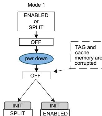
Mode 1 can also be used when the system is in GPRAM mode, but software must take into account that the data in the GPRAM is lost when the system is set in retention.
