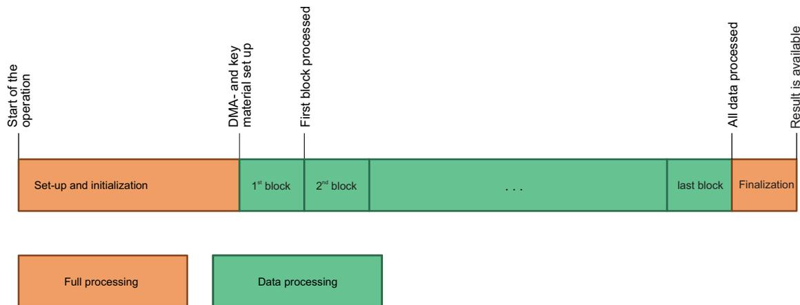
The full processing part is required once per processing command, and precedes the processing of the first data block. The data processing blocks depend on the amount of data to be processed by the command. The finalization is required when the operation produces a result digest or TAG.
