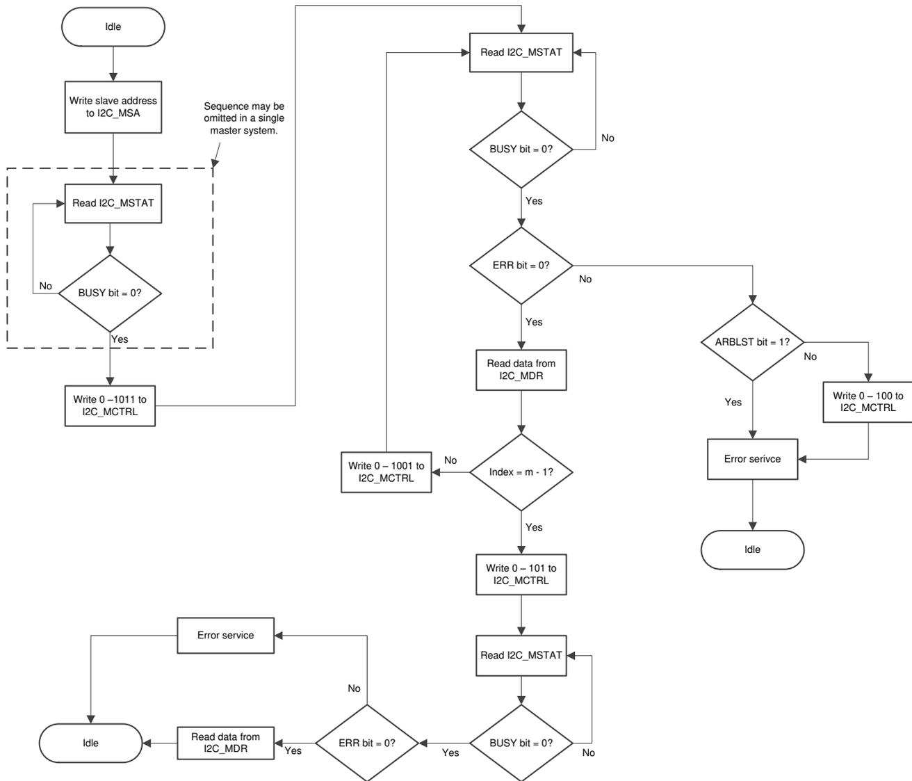
Figure 21-11. Master RECEIVE With Repeated Start After TRANSMIT With Repeated Start Condition
