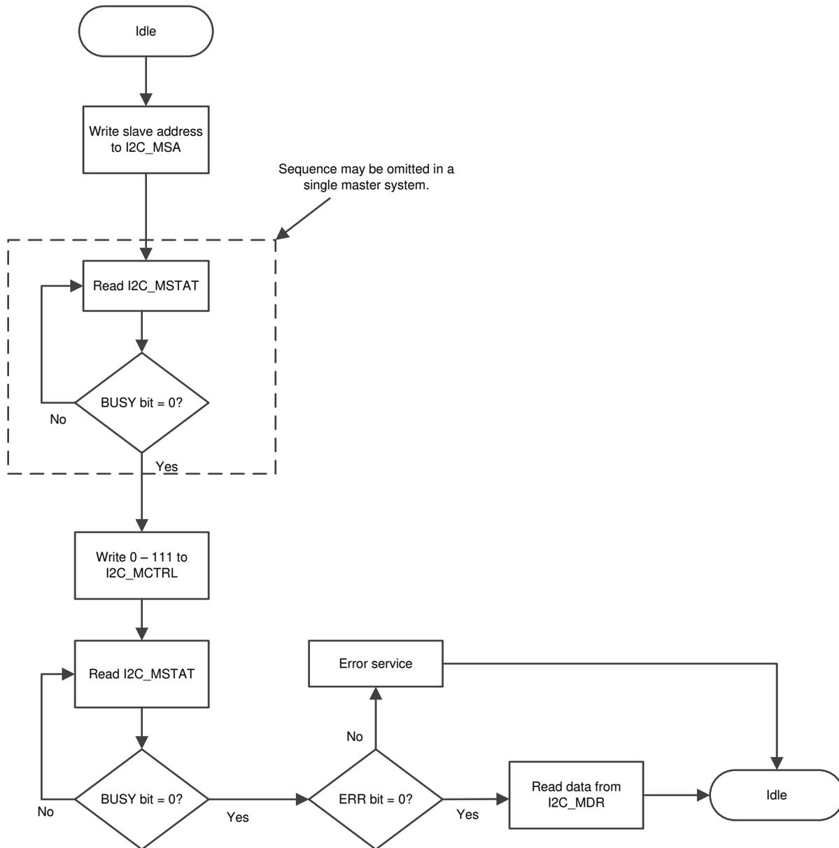
Figure 21-9. Master TRANSMIT With Repeated Start Condition
