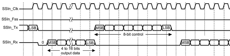
In the MICROWIRE mode, the SSI slave samples the first bit of receive data on the rising edge of SSIn\_CLK after SSIFss has gone low. Masters driving a free-running SSIn\_CLK must ensure that the SSIFss signal has sufficient setup and hold margins compared to the rising edge of SSIn\_CLK.
