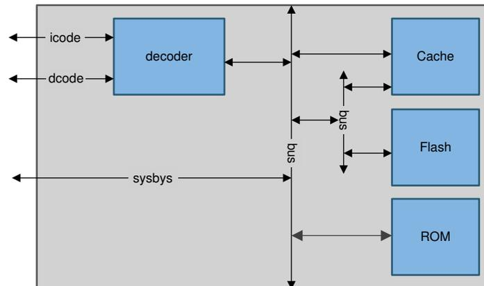
The VIMS module forwards CPU accesses (icode/dcode) and system bus accesses to the addressed memories; the VIMS module also arbitrates access between the CPU and the system bus.
