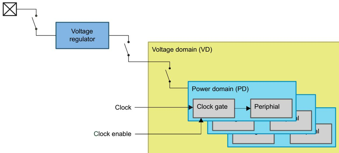
Figure 6-1 shows the hierarchy of power-saving features in the CC26x0 and CC13x0 devices. Low-power consumption and cycling time for a power-saving mode is inversely proportional. The power-saving mode with the lowest power consumption requires the longest time from initiation to power-saving mode, as well as wake-up time back to active mode. Table 6-1 summarizes the power-saving features.
