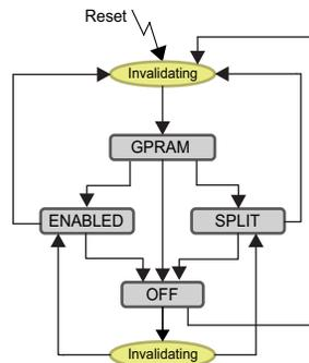
Once a mode change is initiated, shown in the VIMS:STATUS.MODE\_CHANGING register, the mode change must complete before another mode change can be initiated. The VIMS:CTL.MODE register is blocked for updates during a mode change.
