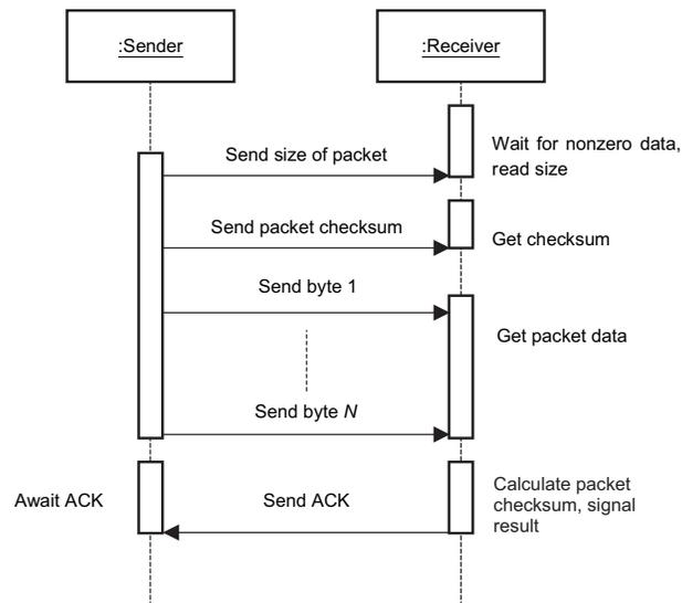
The following steps must be performed to successfully send a packet:
