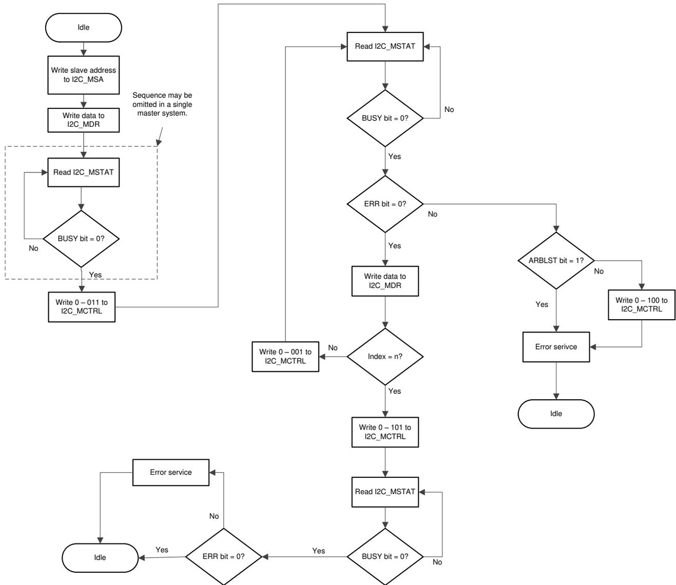
Figure 21-10. Master RECEIVE With Repeated Start Condition
