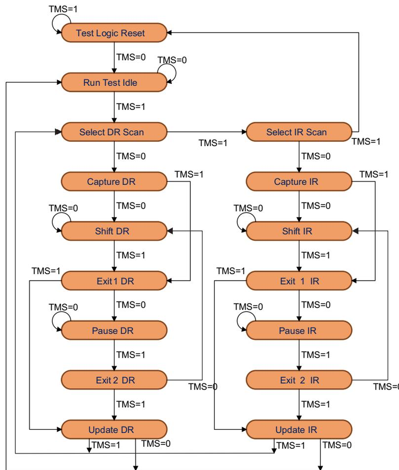
Every state has two exits, so all transitions can be controlled by the single TMS signal sampled on TCK. The two main paths allow for setting or retrieving information from either a data register (DR) or the instruction register (IR) of the device. The data register depends on the value loaded into the instruction register.
