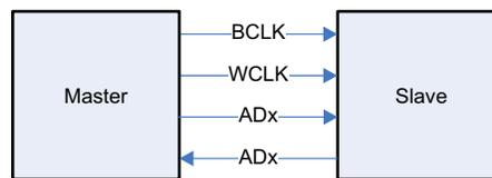
The supported interface formats are synchronous to the BCLK, and the words (samples) are aligned according to the WCLK signal. WCLK is synchronous to BCLK signal, and for all supported interface formats, the frequency of WCLK is the same as the sample frequency. The period from one positive WCLK edge to the next positive WCLK edge is called a frame. Depending on the interface format, a frame may consist of one or two phases.
