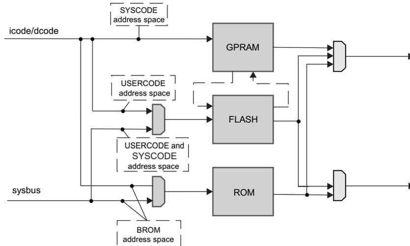
In cache mode, all CPU accesses to the flash SYSCODE address space are directed to the cache first. The cache looks up the input address in the internal tag RAM to determine whether the access is a cache hit or a cache miss.
