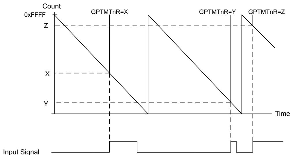
**NOTE:** When operating in edge-time mode, the counter uses a modulo  $2^{24}$  count if prescaler is enabled, or  $2^{16}$  if prescaler is not enabled. If there is a possibility the edge could take longer than the count, another timer can be used to ensure detection of the missed edge.
