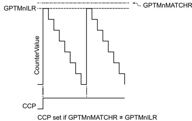
Figure 13-6 shows how the CCP output operates when the PLO and MRSU bits are set and the GPT:TnMATCHR register value is the same as the GPT:TnILR register value. In this situation, if the PLO bit is 0, the CCP signal goes high when the GPT:TnILR register value is loaded, and the match would be essentially ignored.
