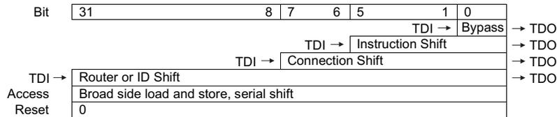
When asked to shift, 1 bit is shifted from each bit into the next lower bit. A new value is shifted in from TDI while the least significant bit is shifted out to TDO. The shift register has several insertion points based on the current TAP state or value in the instruction register.
