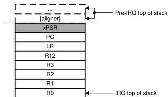
Immediately after stacking, the stack pointer indicates the lowest address in the stack frame.
