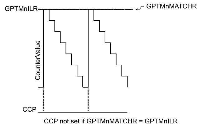
Figure 13-7 shows how the CCP output operates when the PLO and MRSU bits are set and the GPT:TnILR register value is greater than the GPT:TnMATCHR register value.
