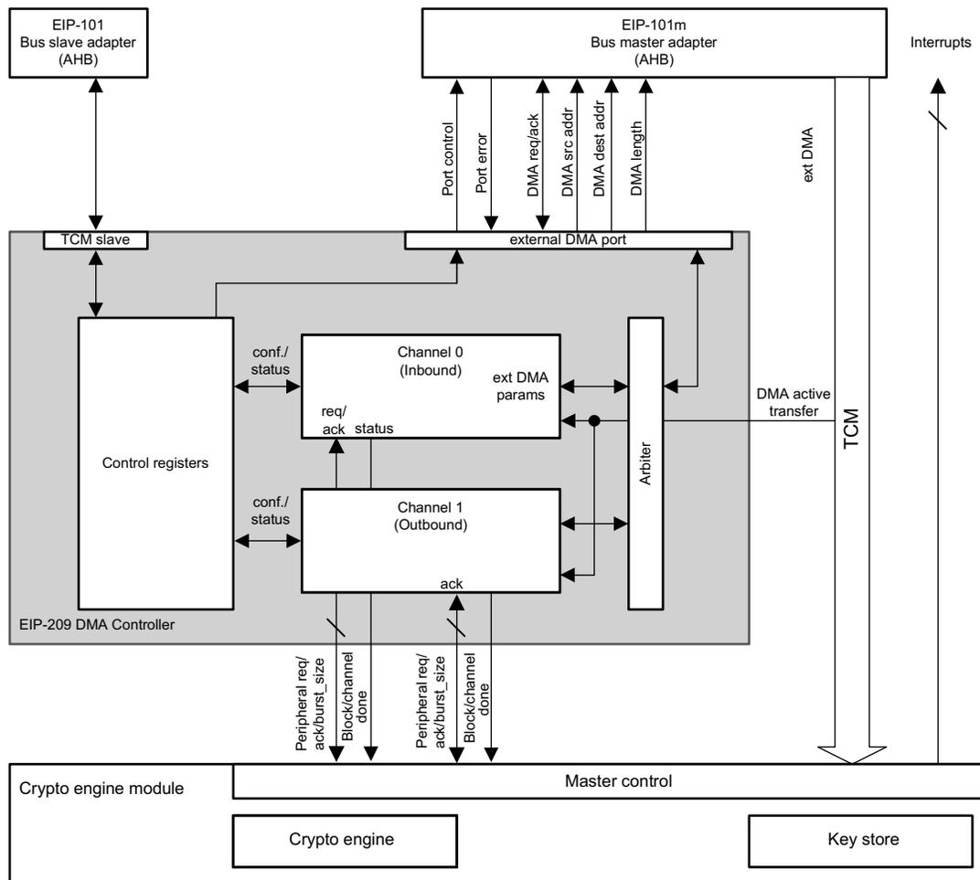
The DMAC of the AES module controls the data transfer requests to the AHB master adapter, which transfers data to and from the AES engines and key store area.
