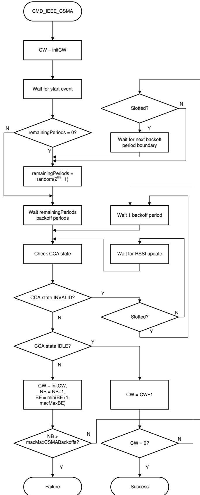
For operation according to IEEE 802.15.4, the parameters must be initialized as follows before starting a new CSMA-CA operation:
