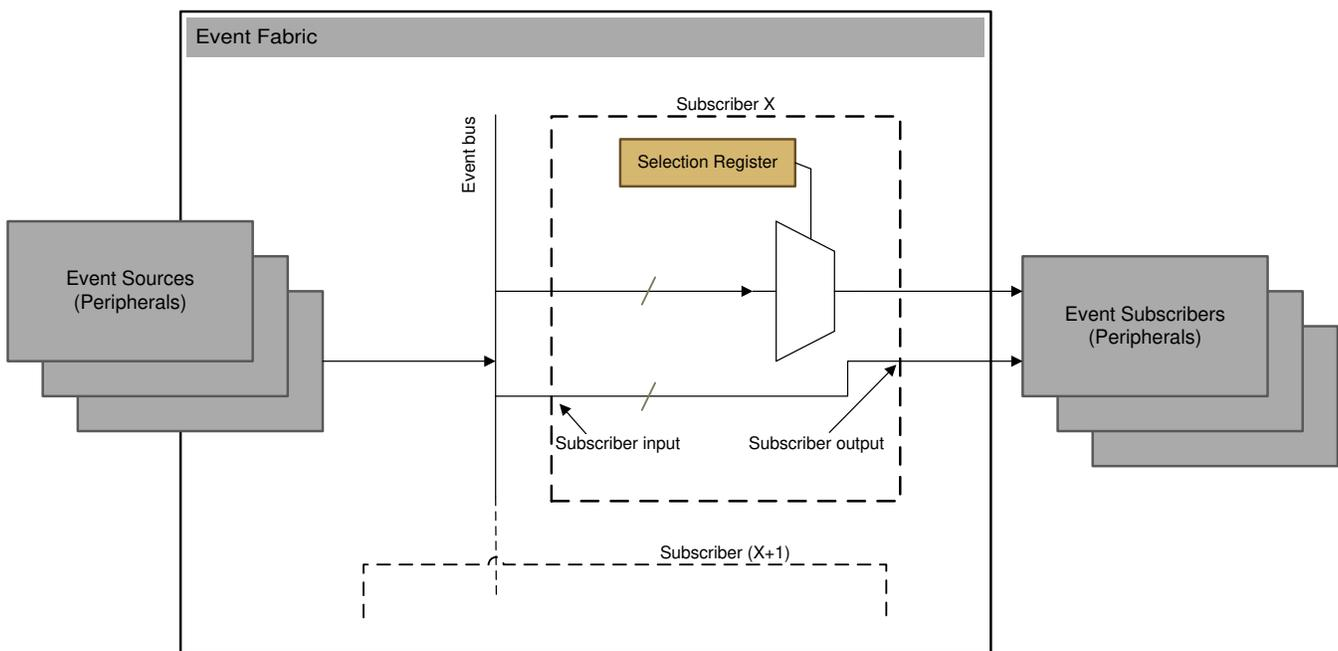
[Figure 4-3](#) shows a simple illustration of the event fabric concept. Clearly the event fabric is not a peripheral in itself, but rather a block of routing between the peripherals and more. The lines that have configurable inputs are controlled by selection registers that are connected to a MUX, which forwards the selected input in the subscriber to the peripherals.
