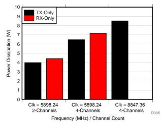
Figure 4. Power Dissipation in TDD Mode
